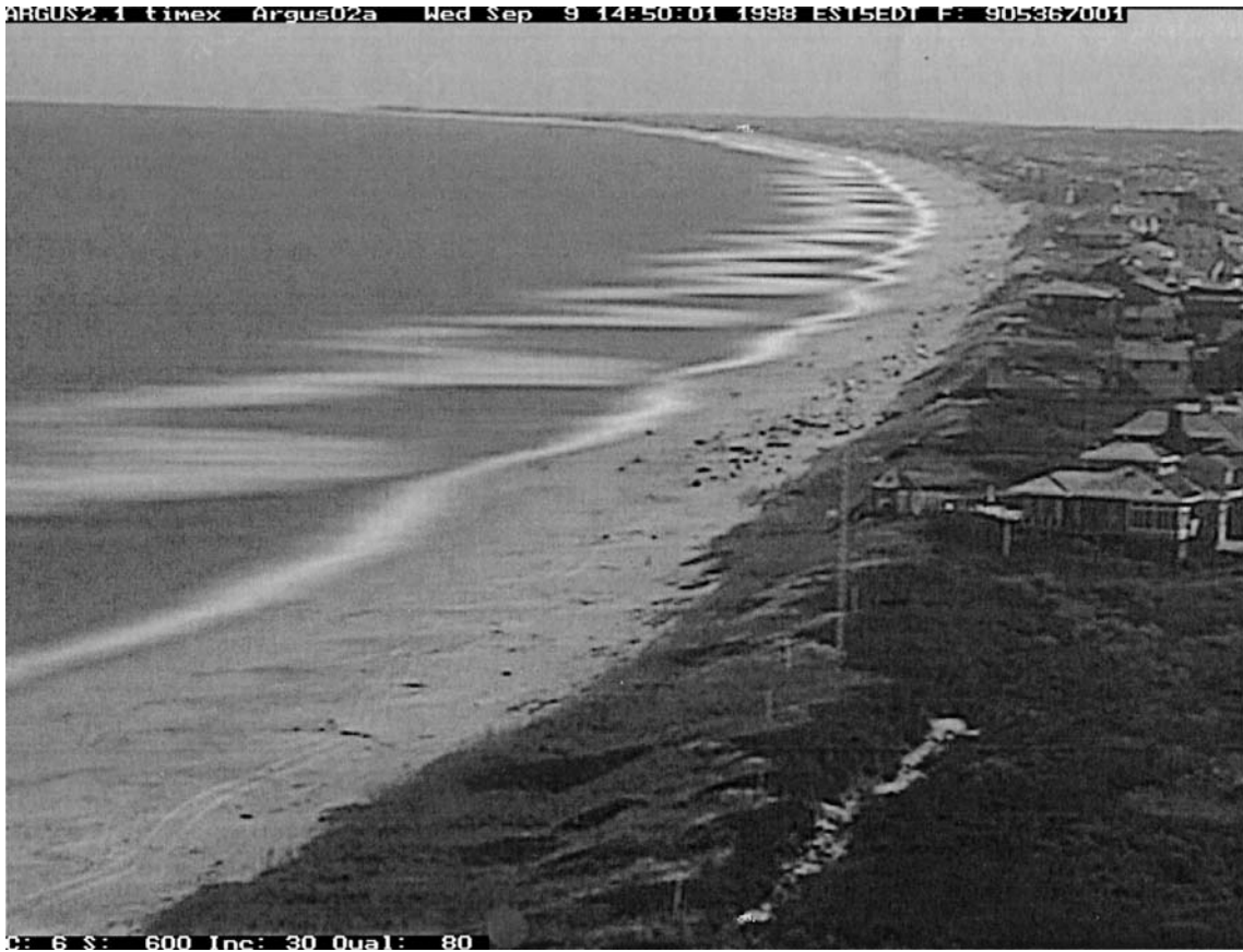
Figure 1. Video image of nearshore morphology (crescentic bars) observed just south of the pier at the U.S. Army Field Research Facility at Duck, North Carolina. The white areas indicate the locations where incoming waves break at the bars. Image reproduced by kind permission of Prof. Rob Holman of Coastal Imaging Lab., College of Oceanic and Atmospheric Sciences, Oregon State University.
