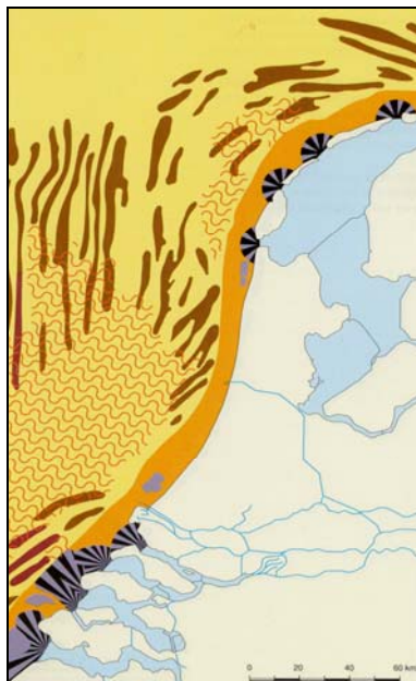
Figure 1: Overview of large-scale seabed patterns in the Dutch part of the North Sea. Dark patches are tidal sandbanks, curly lines indicate sandwave fields. Source: Van Alphen & Damoiseaux [1989].
