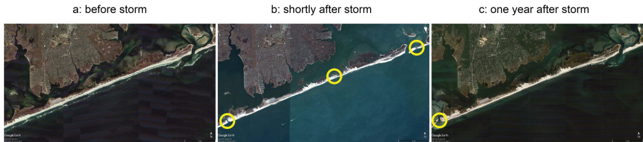
Figure 3.1: Satellite images of three storm-induced breaches at Fire Island and Westhampton (Long Island, NY, USA) due to hurricane Sandy in 2012 showing: a, before the storm (07-March-2012); b, shortly after the storm (04-November-2012); c, almost one year after the storm (20-September-2013). The location of the breaches is indicated with yellow circles (Google, 2016, Map Data: DigitalGlobe, USDA Farm Service Agency).
