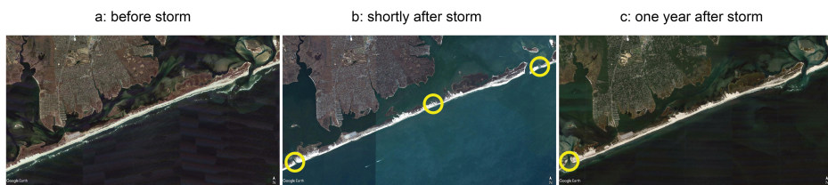
Figure 1.6: Satellite images of three storm-induced breaches at Fire Island and Westhampton (Long Island, NY, USA) due to hurricane Sandy in 2012 showing: a, before the storm (07-March-2012); b, shortly after the storm (04-November-2012); c, almost one year after the storm (20-September-2013). The location of the breaches is indicated with yellow circles. Retrieved from Google Earth (Map Data: DigitalGlobe, USDA Farm Service Agency). Image used with permission from Reef et al. (2020b).
