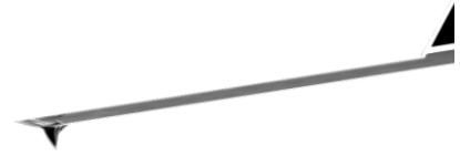
**Figure 1:** Cantilever. 228  $\mu\text{m}$  long silicon cantilever with integrated tip.
