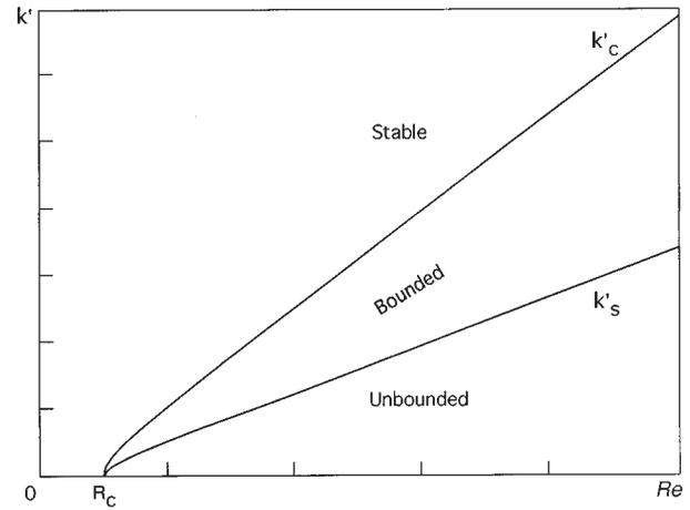
FIG. 37. Phase diagram for the Benney equation (6.2).  $R_c = \frac{5}{3} \cot \theta$  is the critical value of the Reynolds number  $Re$ . For  $Re < R_c$  the state  $H=1$  is stable. If  $Re > R_c$  then (i) for  $k' < k'_s$  two-dimensional waves blowup in a finite time; (ii) for  $k'_s < k' < k'_c$  two-dimensional waves saturate; (iii) for  $k' > k'_c$  initial perturbations of  $H=1$  decay. Here  $k'_c = [\frac{2}{155} Re(Re - R_c)]^{1/2}$  and  $k'_c = 2k'_s$ .
