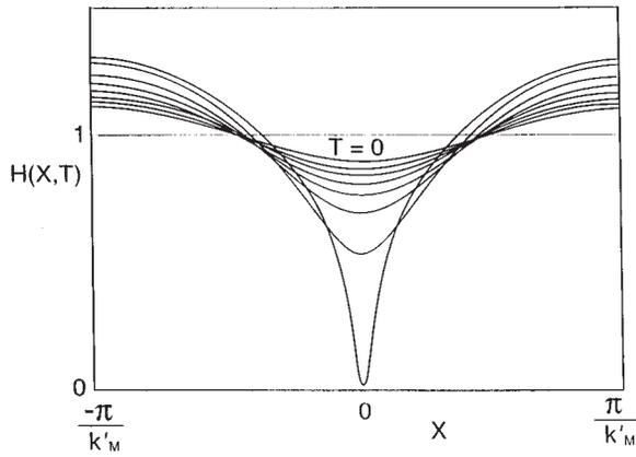
FIG. 12. Film profiles at different times as given by Eq. (2.41b) for  $A = C^{-1} = 1$  solved in the domain  $-\pi/k_M \leq X \leq \pi/k_M$  with the initial condition  $H(X, T=0) = 1 + 0.1 \sin(k_M X)$ . The fastest-growing linear mode has a wave number  $k_M$ ,  $2k_M^2 = 1$ . Copyright © 1988 Cambridge University Press. Reprinted with the permission of Cambridge University Press from Burelbach, Bankoff, and Davis (1988).
