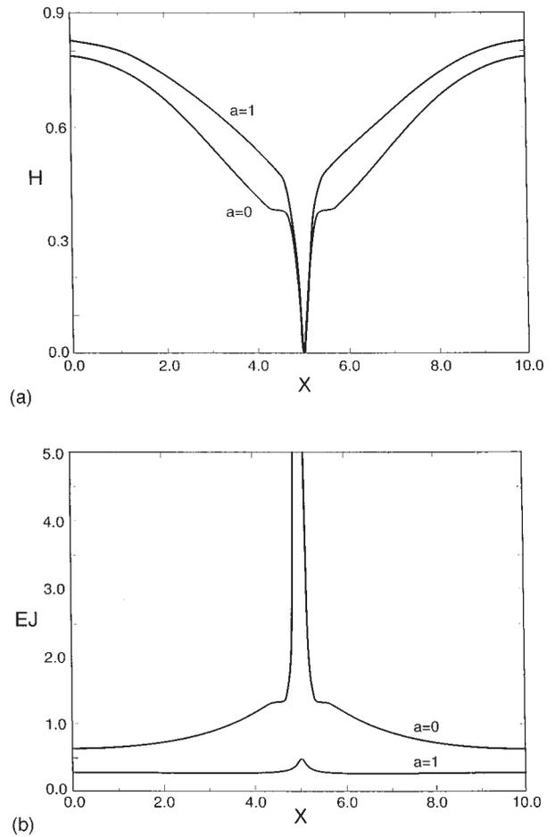
FIG. 19. Film profiles for rupture with evaporation. (a) The film interface at rupture for  $a=0$  and  $a=1$ , as given by Eq. (2.91) with  $A=1, K=0, \bar{E}=0.5, \bar{C}^{-1}=1$ , (b) the evaporative mass flux  $J = \bar{E}(H+a)^{-1}$  along the film interface, as calculated for the two cases shown in (a).
