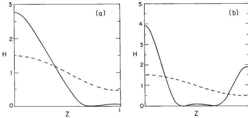
FIG. 20. Quasisteady long-time behavior of an annular film, Eq. (2.103a): (a)  $\Delta = 2^{3/2}\pi$ ; (b)  $\Delta = 6\pi$  and  $Z = 2X/\Delta$ . Initial disturbances are represented by the dashed lines. The pressure within each of the lobes is almost constant; the small lobes are slowly draining into their larger neighbors. Only half a period is shown. Copyright © 1983 Cambridge University Press. Reprinted with the permission of Cambridge University Press from Hammond (1983).
