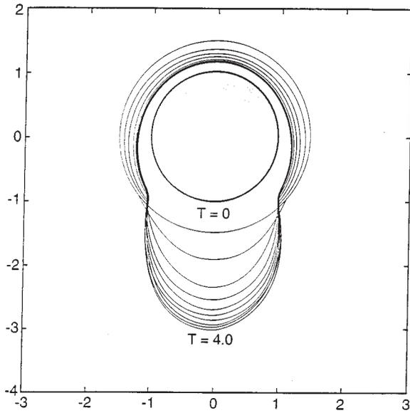
FIG. 23. Unsteady film flow for an isothermal film on a horizontal cylinder,  $Bo^{-1}=0.25, A=0$ . Copyright © 1992 Cambridge University Press. Reprinted with the permission of Cambridge University Press from Reisfeld and Bankoff (1992).
