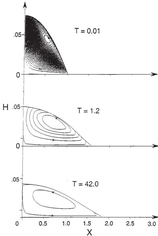
FIG. 34. Nonisothermal spreading: evolution of the stream function with  $\hat{M}=0.2, \theta_A=0.25, B \ll 1$ , and  $G=0$ . Instantaneous streamlines are given in steps of  $\Delta\psi=0.01$ . Copyright © 1991 Cambridge University Press. Reprinted with the permission of Cambridge University Press from Ehrhard and Davis (1991).
