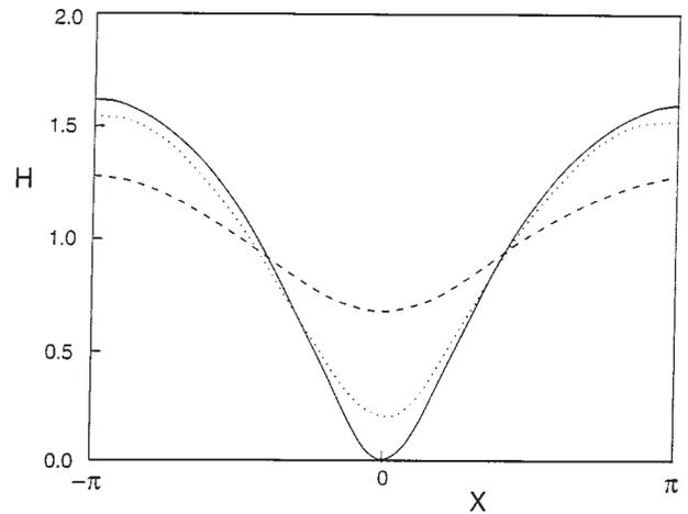
FIG. 27. Dimensionless steady layer profile  $H(X)$  for various values of  $B_{\text{dyn}}$ , for a fixed value of  $\bar{C}^{-1}/G = 0.6174$ , calculated from Eq. (3.5) with  $\Theta_b(X) = \frac{1}{2}\cos X$  and  $B = 0$ ; dashed line,  $B_{\text{dyn}} = 0.627$ ; dotted line,  $B_{\text{dyn}} = 1.255$ ; solid line  $B_{\text{dyn}} = 1.445$ . Reprinted with the permission of the American Institute of Physics from Tan *et al.* (1990).
