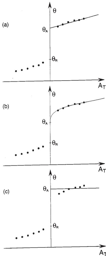
FIG. 32. Typical measurements of contact angle after Dussan V. (1979).  $\partial_T A \equiv u_{CL}$  is the speed of the contact line. Symbols represent experimental data, solid lines correspond to various mobility exponents  $m$  in the model of Eqs. (5.8): (a)  $m=1$ ; (b)  $m=3$ ; (c)  $m=\infty$ . Copyright © 1991 Cambridge University Press. Reprinted with the permission of Cambridge University Press from Ehrhard and Davis (1991).
