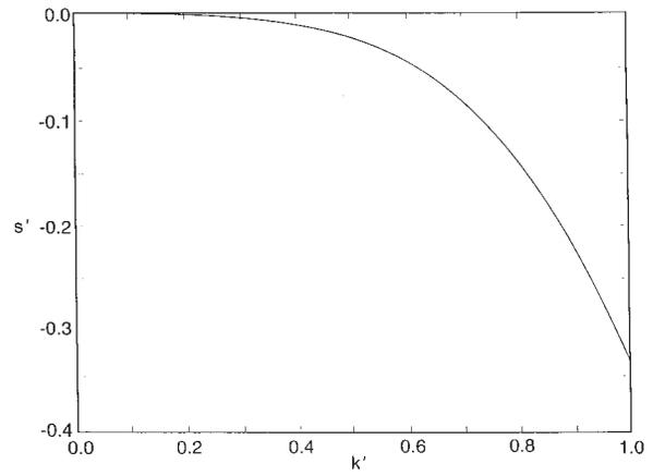
FIG. 8. Characteristic equation given by Eq. (2.35).  $s' = \text{Re}(s)h_0\mu/\sigma$  is the dimensionless growth rate of the perturbation with the dimensionless wave number  $k'$ . Negative growth rate corresponds to the decay of a perturbation; therefore there is no instability ( $s' > 0$ ) in the system.
