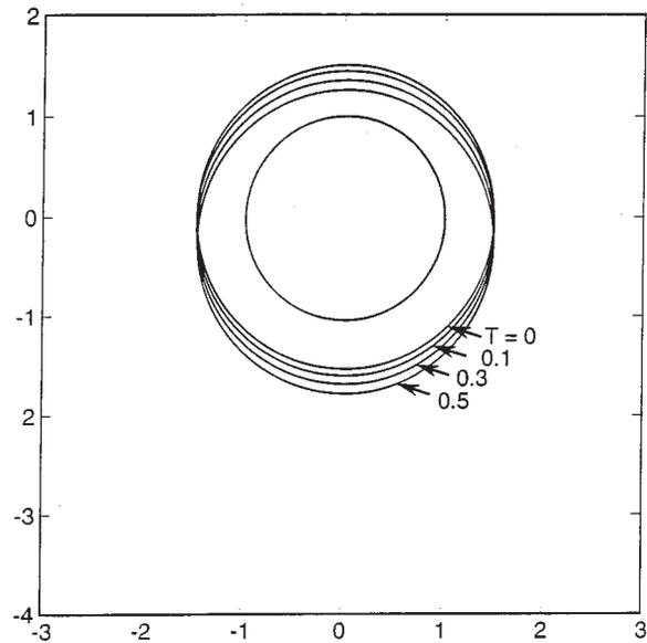
FIG. 22. Unsteady film flow for an isothermal film on a horizontal cylinder,  $Bo^{-1}=0, A=0$ . Copyright © 1992 Cambridge University Press. Reprinted with the permission of Cambridge University Press from Reisfeld and Bankoff (1992).
