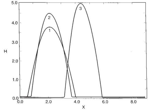
FIG. 14. Steady-state solutions for a film under the simultaneous action of attractive and repulsive intermolecular forces, as described by Eq. (2.47a) with  $G=0$  and  $\Phi_0 = H^{-3} - \bar{a}_4 H^{-4}$  [the dimensionless version of Eq. (2.48e)]. Curve 1,  $\bar{a}_4 = 0.1, \bar{C}^{-1} = 1$ ; Curve 2,  $\bar{a}_4 = 0.1, \bar{C}^{-1} = 0.05$ ; Curve 3,  $\bar{a}_4 = 0.05, \bar{C}^{-1} = 1$ .
