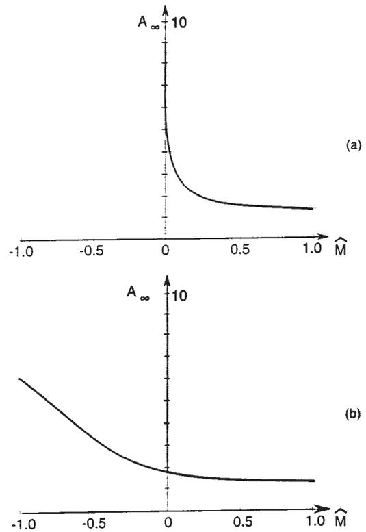
FIG. 33. Final spreading: final drop widths  $A_\infty$  as functions of Marangoni number  $\hat{M}$  for  $G=0$  and  $B \ll 1$ , for two different advancing contact angles: (a)  $\theta_A=0$ ; (b)  $\theta_A=0.5$ . The curves are obtained from Eq. (5.21). Copyright © 1991 Cambridge University Press. Reprinted with the permission of Cambridge University Press from Ehrhard and Davis (1991).
