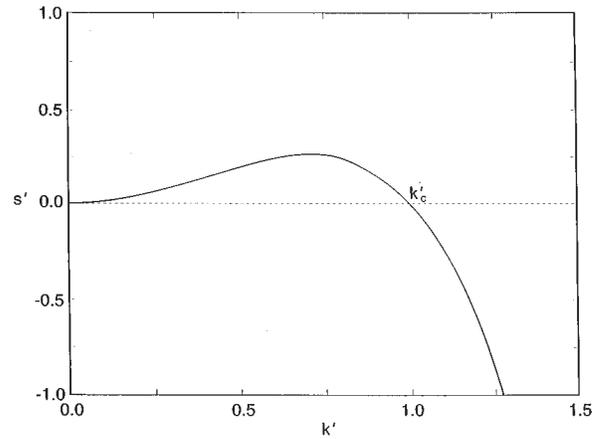
FIG. 10. Characteristic equation given by Eq. (2.38) for the Bond number  $Bo = 1$ , as defined by Eq. (2.39).  $s' = 3s\mu/\rho|g|h_0$  is the dimensionless growth rate of the perturbation with the dimensionless wave number  $k'$ . Positive growth rate corresponds to the growth of a perturbation, whereas negative growth rate indicates decay. Therefore the unstable domain is  $0 < k' < k_c'$ .
