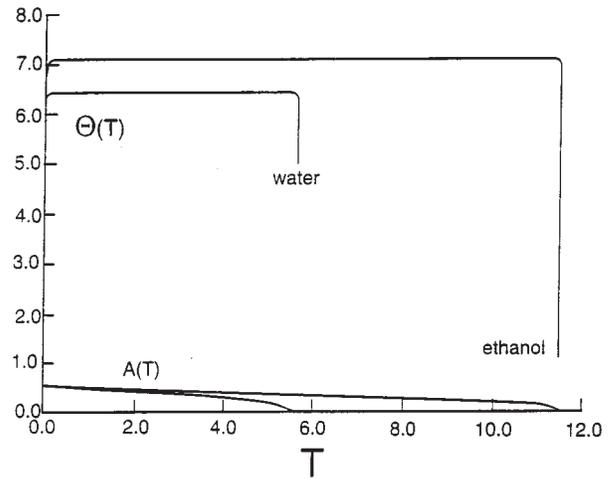
FIG. 35. The angle  $\theta$  and the location of the contact line  $A$  in a spreading drop as functions of time  $T$ . Reprinted with the permission of the American Institute of Physics from Anderson and Davis (1995).
