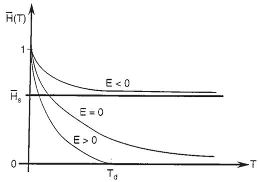
FIG. 26. Basic-state film thickness for principal values of the evaporation number  $E$  for rotating liquid films. Reprinted with the permission of American Institute of Physics from Reisfeld *et al.* (1991).
