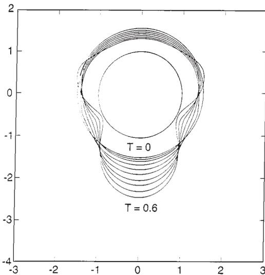
FIG. 24. Unsteady film flow and rupture for a heated film with  $Bo^{-1}=0.1, M/P_r Gr=5$ . Copyright © 1992 Cambridge University Press. Reprinted with the permission of Cambridge University Press from Reisfeld and Bankoff (1992).
