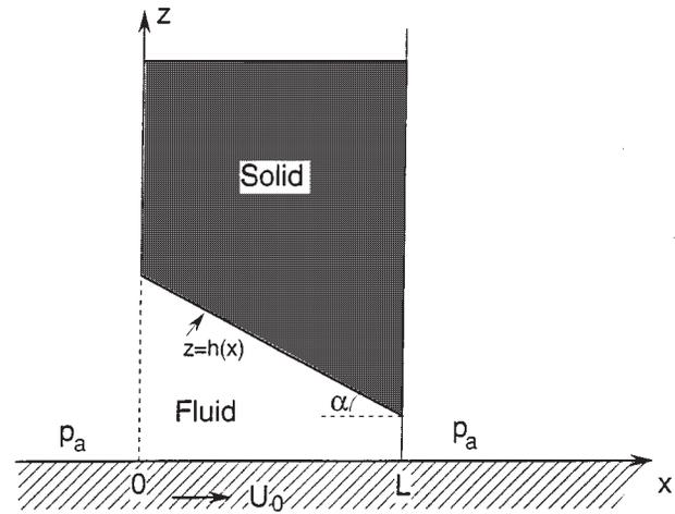
FIG. 5. Slipper bearing. The plate moves with the constant velocity  $U_0$ . The lower boundary of the bearing, located at  $z=h(x)$ , is static and tilted at small angle  $\alpha$ . The external pressure is  $p_a$ .
