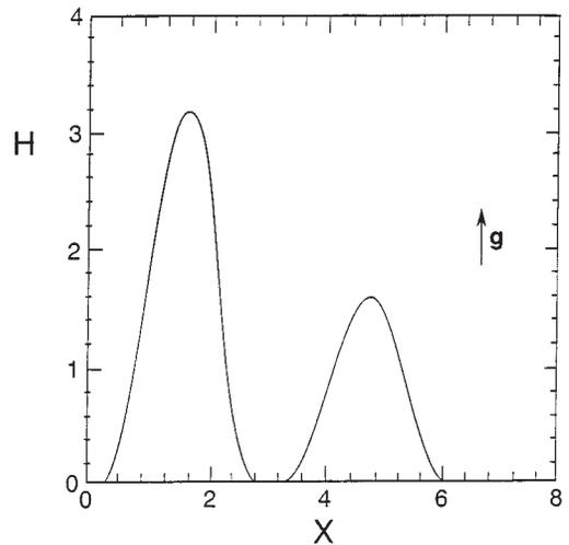
FIG. 11. Film profile close to rupture for Rayleigh-Taylor instability for  $G = 20$ ,  $C^{-1} = 4$ ,  $\Delta = 2\pi$ , and the initial condition  $H(X, T = 0) = 1 + 0.005 \sin X$ . The arrow indicates the direction of gravity.
