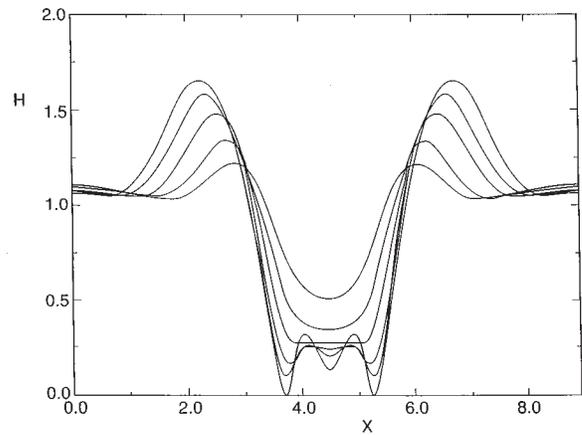
FIG. 28. Evolution of the dimensionless layer profile  $H(X)$  for a film heated by spatially nonuniform heat flux. The evolution is described by Eqs. (3.9) and (3.11), with  $E=0, A=1, G=0, C^{-1}=1, a=1, D^{-1}=0, MKP_r^{-1}/2=40$ . A satellite drop splits into two partially coalesced drops.
