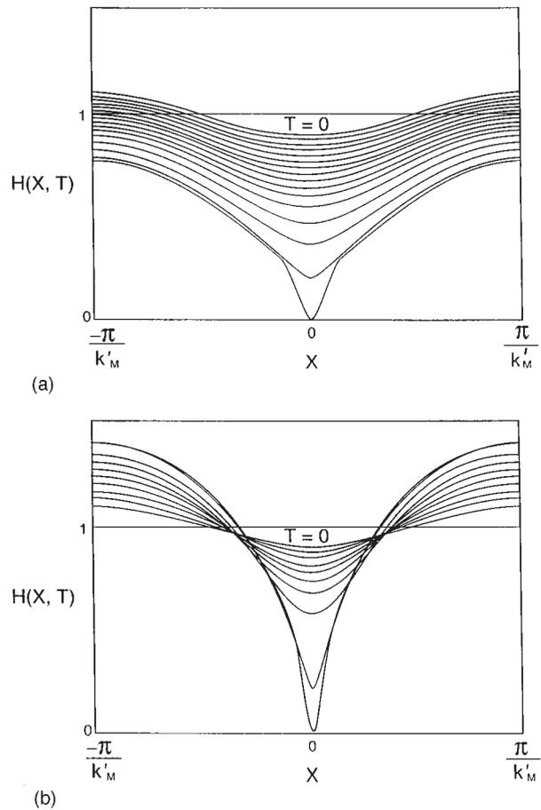
FIG. 17. Film profiles at different times: (a) quasiequilibrium evaporation, when vapor recoil and mass loss are both important,  $A=1, \bar{C}^{-1}=1, K=0, \bar{E}=1, D=1$ ; (b) nonequilibrium condensation including mass gain, vapor recoil, and thermocapillarity,  $\bar{E}=-0.1, \bar{E}^2 D^{-1}=1, MP_r^{-1}=-1, A=1, \bar{C}^{-1}=1, K=0.1$ . Copyright © 1988 Cambridge University Press. Reprinted with the permission of Cambridge University Press from Burelbach, Bankoff, and Davis (1988).
