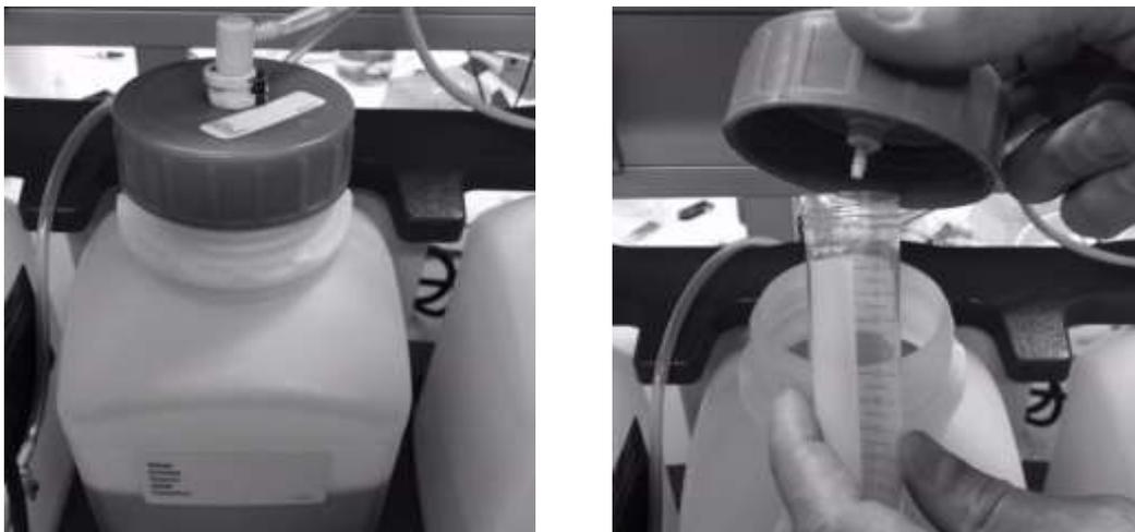
Figure 2 Manual waste collection from the CellSearch Autoprep by unscrewing the top from the waste container (left) and collecting the sample in a 50 mL Greiner tube.
