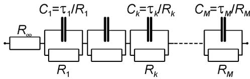
**Figure 1:** Arrangement of the series of (RC) circuits used in the Kramers-Kronig data validation test.
