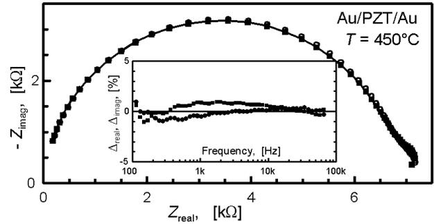
**Figure 2:** Impedance spectrum for a non-equilibrium measurement. Insert shows the traces of the residuals (comparison between data and KK-fit using eq. (5)).
