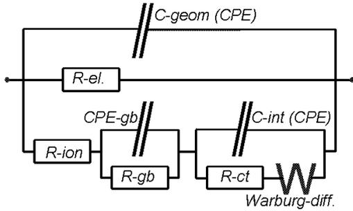
**Figure 6:** Equivalent circuit that has been assembled during the subtraction procedure. This circuit has been used in the CNLS-fit presented in Fig. 3.
