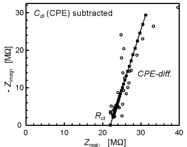
**Figure 5:** Remaining electrode dispersion after subtraction of the bulk ionic contribution and the double layer capacitance (CPE) from the dispersion of Fig. 4. Solid squares are a fit to the data points.
