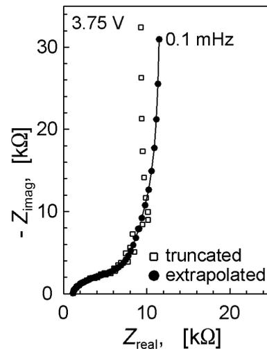
**Figure 7:** Diffusion impedance of Li-insertion in a  $\text{Li}_x\text{CoO}_2$  cathode. Transformation from a time-domain measurement with a voltage step of 10 mV [11].
