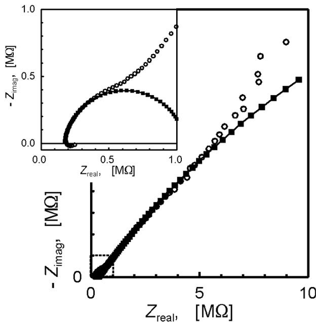
**Figure 4:** Impedance diagram after subtraction of the dielectric response and the electronic conductivity. Insert shows enlargement of the high frequency part. Solid squares present the partial  $R(RQ)$  fits, see text.
