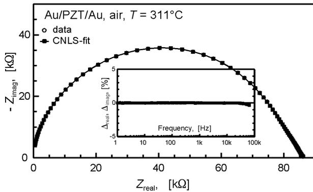
**Figure 3:** Impedance of a PZT sample with gold electrodes. Both data points and CNLS-fit are presented. The insert shows the distribution of the residuals.
