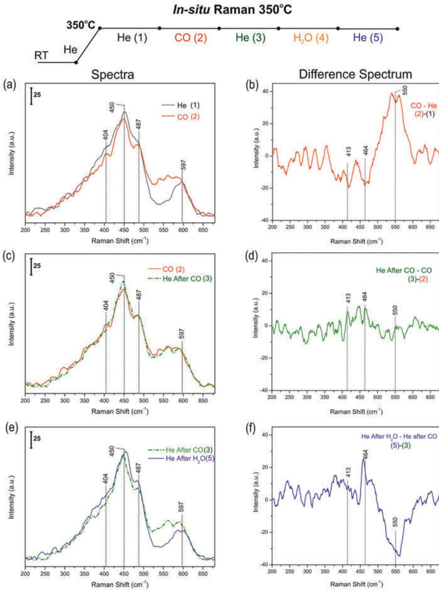
**Figure 4.5:** *In situ* Raman spectra at 350°C of ceria rods a) in He(1) (black solid spectrum), followed by CO(2) (red solid line); b) CO(2) - He(1); c) CO(2) (red solid line) followed by He(3) (green dash-dotted line); d) He(3) - CO(2); e) He(3) and He(5) after He/H<sub>2</sub>O(4) flow (blue solid spectrum); f) He(5) - He(3).
