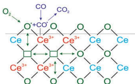
**Figure 1.11:** Catalytic pathway for CO oxidation on CeO<sub>2</sub> rods. Adapted from Reference[93]
