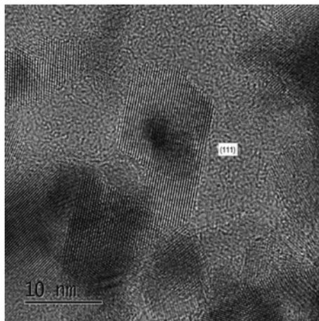
**Figure A2.2:** AC-TEM image of CeO<sub>2</sub> octahedra showing that the smaller particles (~ 1 nm) also expose prominent (111) facets. The shapes are not as well defined as the larger octahedra imaged by HRSEM (figures 2.2 and 2.3). The exposure of two parallel (111) surfaces with the other surfaces being irregular is also a common feature, and it is expected that the rod cross section also has this same characteristic.
