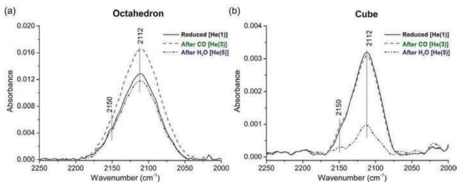
**Figure 5.5:** *In situ* FTIR of reduced ceria (a) octahedra and (b) cubes at 350°C obtained in He(1), He(3) and He(5) flow. Key: He(1) black solid line is obtained for the freshly reduced samples in He flow, He(3) dashed green line is obtained in He flowed after exposure to CO gas and He(5) dash-dotted blue line is recorded in He flow after exposure to H<sub>2</sub>O vapor.
