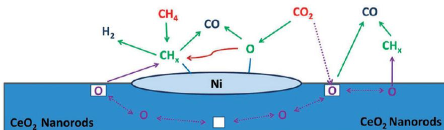
**Figure 1.12:** Catalytic mechanism for CO<sub>2</sub> reforming of methane over Ni-supported CeO<sub>2</sub> rod.[97]
