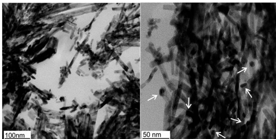
**Figure A2.4:** TEM images of microtomed sections of  $\text{CeO}_2$  rods embedded in epoxy. These sections provide an opportunity to see the rods end-on. The image on the right shows some of the rods end-on (i.e. those with a short aspect ratio), allowing us to image the rods in cross-section. Since the rods are thick when viewed end-on, it is not possible to obtain HRTEM images.
