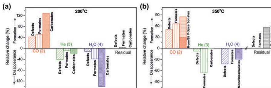
**Figure 4.9:** Bar diagram of species formed (positive) and decomposed (negative values) on introduction different gases in ceria rods at 200°C and 350°C. The numbers represent the relative change (%) for each individual species.
