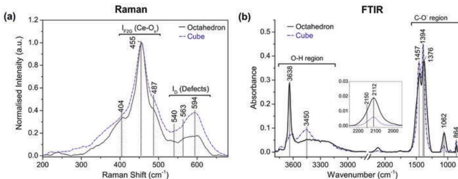
**Figure 5.2:** *In situ* normalized Raman (a) and FTIR (b) spectra of H<sub>2</sub> reduced ceria octahedra (solid black spectrum) and cubes (dash-dotted blue spectrum) in He flow at 350°C.
