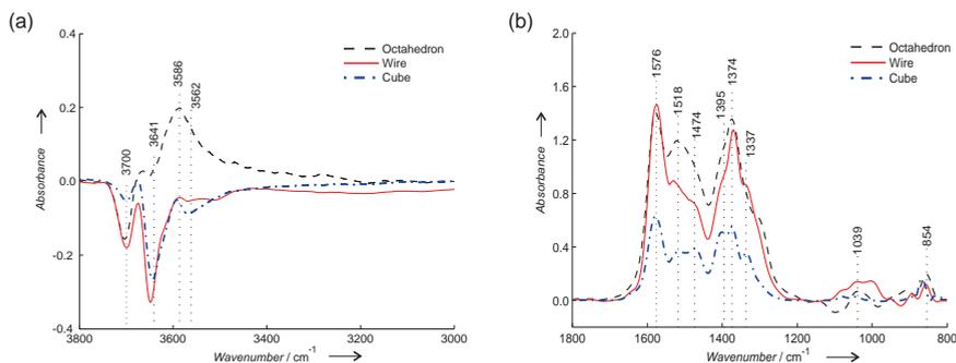
**Figure 3.8:** The He subtracted CO spectra at 200°C of ceria nanoshapes for (a) the hydroxyl region (3800 – 3000 cm<sup>-1</sup>), (b) the C-O<sup>-</sup> region (1800 – 800 cm<sup>-1</sup>).
