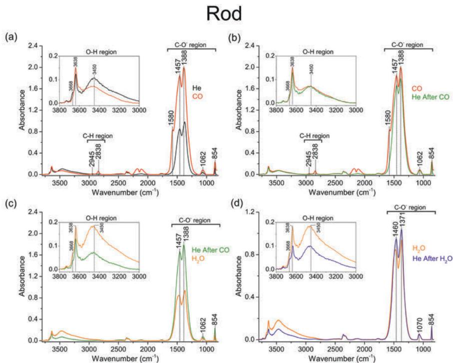
**Figure A5.4:** *In situ* FTIR spectra at 350°C of reduced ceria rods in a) He(1, black spectrum), followed by CO(2, red line); b) CO(2) followed by He(3, green spectrum); c) He(3) followed by H<sub>2</sub>O/He(4, orange line); d) in H<sub>2</sub>O(4) followed by He(5, blue spectrum).
