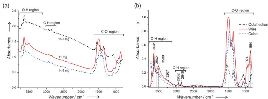
**Figure 3.4:** *In situ* FTIR (a) raw and (b) baseline corrected spectra of ceria cubes (dashed blue), wires (solid red) and octahedra (dash-dotted black spectrum) at 200°C in He flow (after 30 min of flow).
