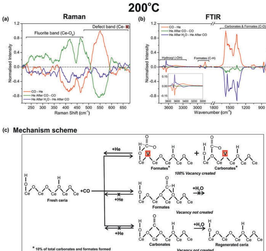
**Figure 4.7:** Relative changes introduced in different gases with respect to the species formed in CO for (a) Raman and (b) FTIR data at 200°C. c) Schematic reaction mechanism of ceria rods at 200°C (“V” represents oxygen vacancy). For simplicity only surface defects are indicated. However, oxygen diffusion will occur through the lattice to reach equilibrium between surface and bulk defects.
