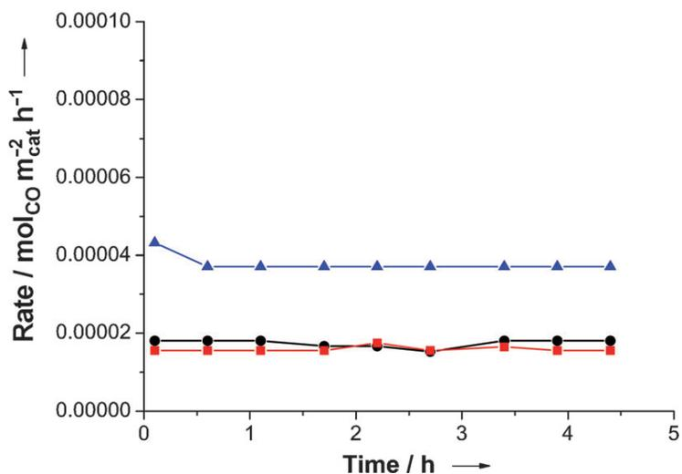
**Figure 2.11:** Rate of CO conversion per m<sup>2</sup> during WGS reaction for rods (red), octahedra (black), and cubes (blue) at 350°C after H<sub>2</sub> pretreatment at 500°C.
