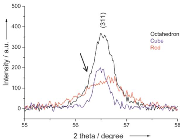
**Figure A2.1:** Expanded view of the (311) reflection in the XRD patterns of the  $\text{CeO}_2$  samples. The peak asymmetry can be clearly seen and the presence of the shoulder on the left (pointed with an arrow) indicates that a portion of the sample has an expanded lattice constant.
