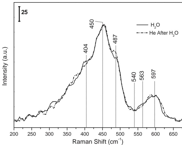
**Figure A4.5:** *In situ* Raman spectra at 350°C of ceria rods in H<sub>2</sub>O/He (4, solid spectrum) followed by He (5, dash-dotted spectrum) flow.
