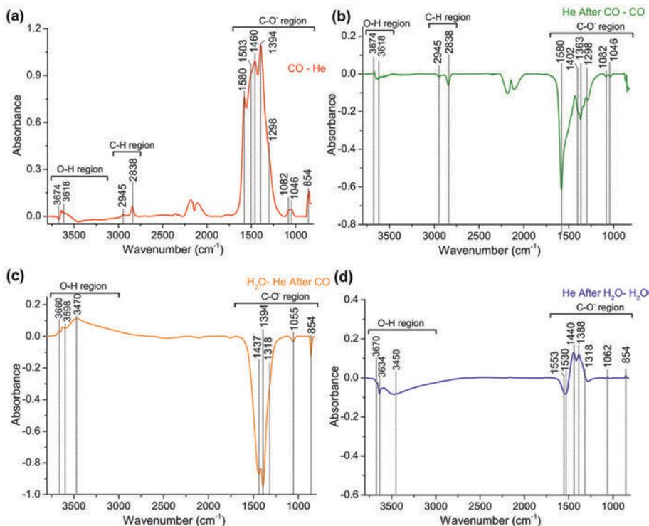
**Figure A5.8:** *In situ* FTIR spectrum of reduced ceria rods at 350°C obtained by subtracting (a) He(1) from CO(2); (b) CO(2) from He(3); (c) He(3) from H<sub>2</sub>O(4); (d) H<sub>2</sub>O(4) from He(5) spectrum.
