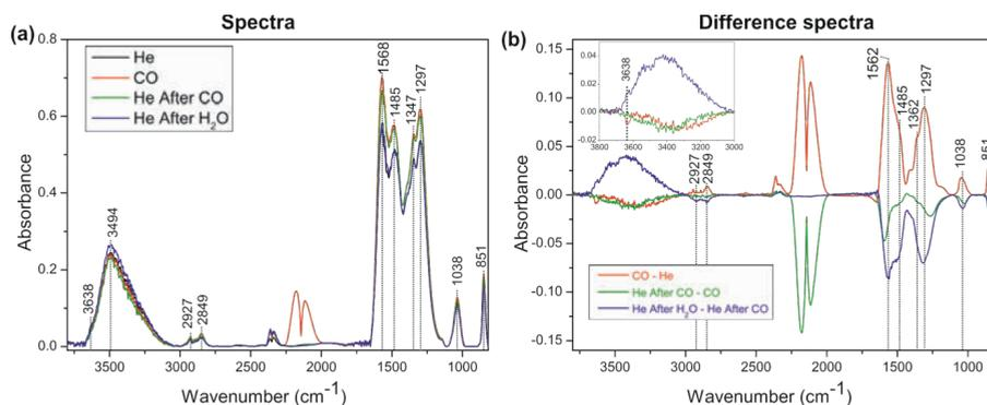
**Figure A4.7:** *In situ* FTIR (a) spectra and (b) difference spectra at 200°C of ceria rods (with KBr) in He flow (black spectrum), followed by 33 vol.% CO/He (red line) and then by He flow (green line) and subsequently in He after H<sub>2</sub>O flow (blue spectrum).
