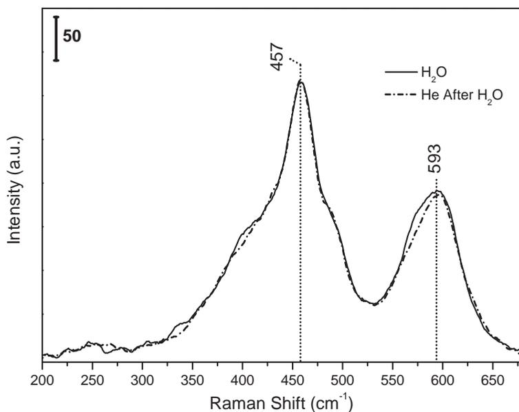
**Figure A4.4:** *In situ* Raman spectra at 200°C of ceria rods in H<sub>2</sub>O/He (4, solid spectrum) followed by He (5, dash-dotted spectrum) flow.
