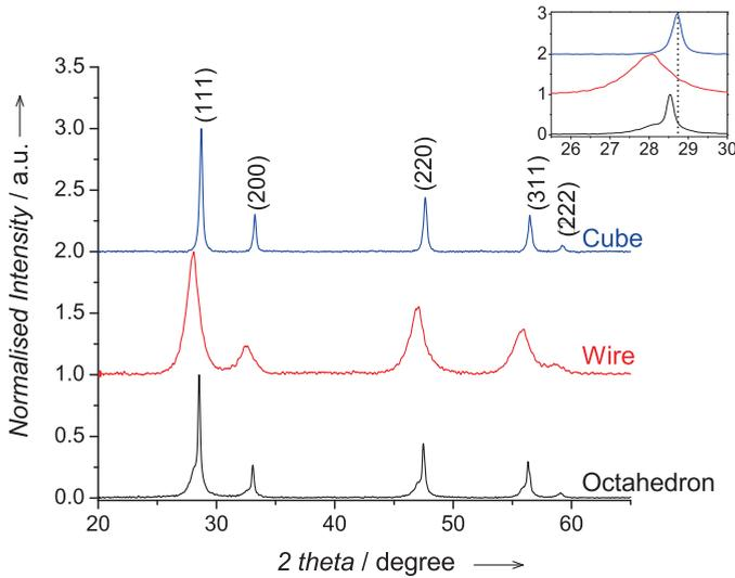
**Figure 3.2:** XRD spectra of the different ceria nanoshapes, normalized to the (111) peaks.
