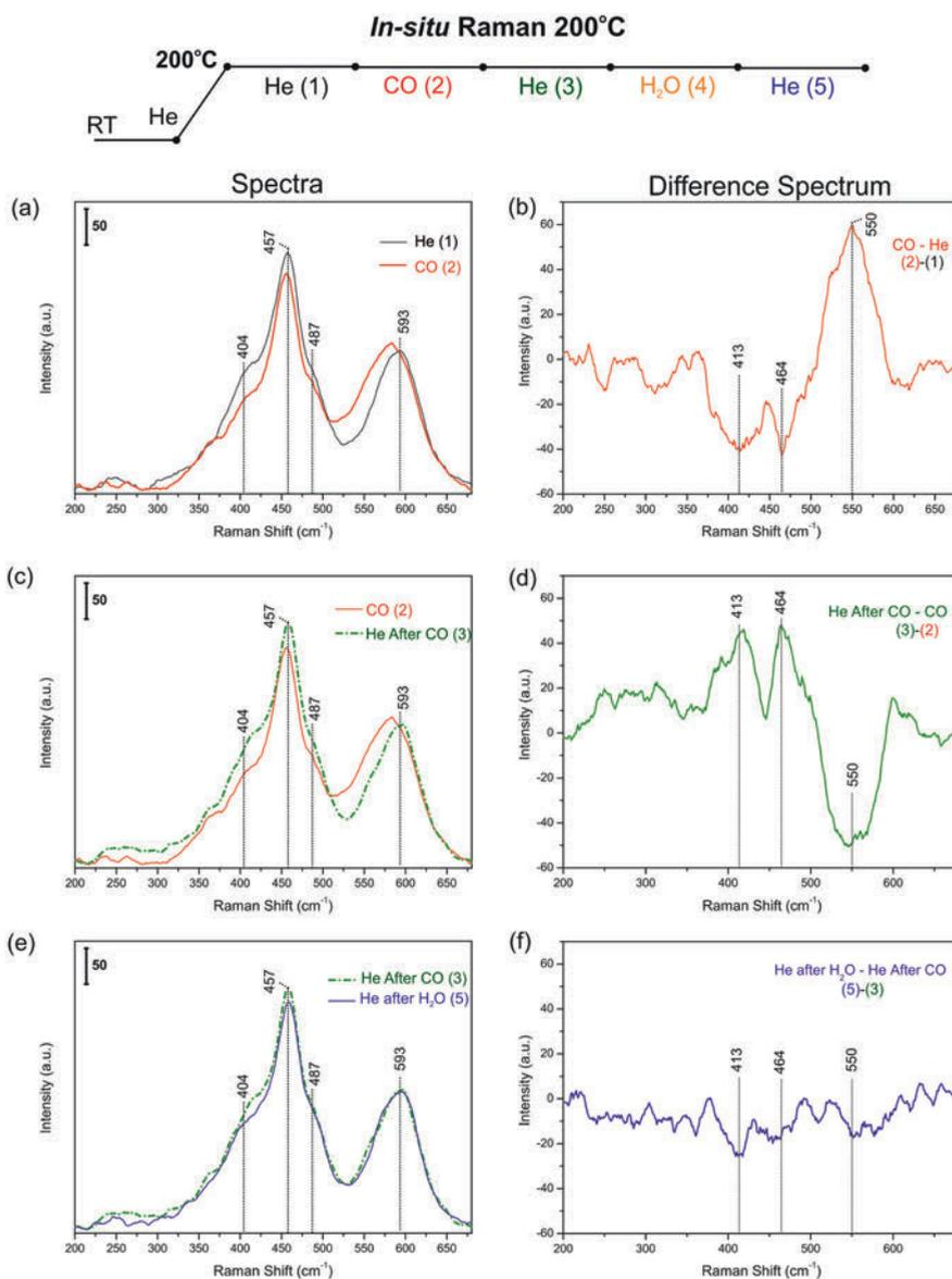
**Figure 4.4:** *In situ* Raman spectra at 200°C of ceria rods a) in He(1) (black solid spectrum), followed by CO(2) (red solid line); b) CO(2) - He(1); c) CO(2) (red solid line) followed by He(3) (green dash-dotted line); d) He(3) - CO(2); e) He(3) and He(5) after He/H<sub>2</sub>O(4) flow (blue solid spectrum); f) He(5) - He(3).
