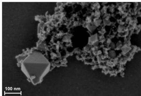
**Figure 2.2:** HRSEM image of the octahedra. Well-defined, faceted octahedra of differing size are present in this sample. This sample shows a distinct bimodal size distribution, with numerous particles that are much smaller than the large octahedra imaged here. This bimodal size distribution gives rise to the asymmetric peaks for the (311) reflection seen in figure A2.1 in the Appendix.
