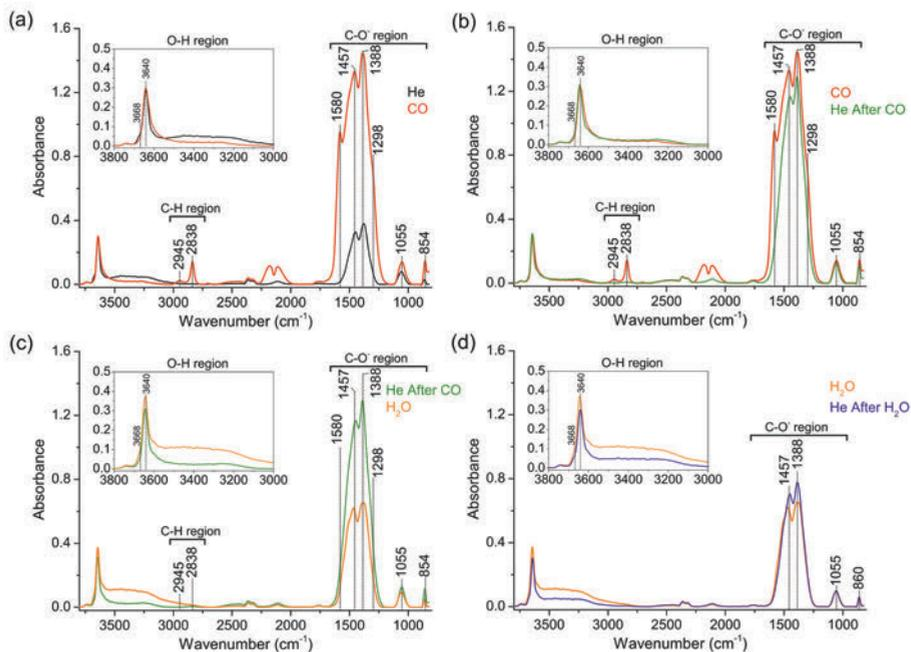
**Figure A5.3:** *In situ* FTIR spectra at 350°C of reduced ceria octahedra in a) He(1, black spectrum), followed by CO(2, red line); b) CO(2) followed by He(3, green spectrum); c) He(3) followed by H<sub>2</sub>O/He(4, orange line); d) in H<sub>2</sub>O(4) followed by He(5, blue spectrum).
