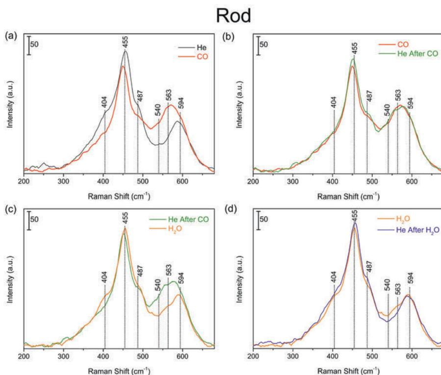
**Figure A5.7:** *In situ* Raman spectra at  $350^\circ\text{C}$  of reduced ceria rods in; (a) He(1, black spectrum), followed by CO(2, red line); (b) CO(2) followed by He(3, green spectrum); (c) He(3) followed by  $\text{H}_2\text{O}/\text{He}$ (4, orange line); (d)  $\text{H}_2\text{O}/\text{He}$  followed by He(5, blue spectrum) flow.
