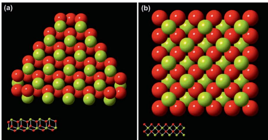
**Figure A2.6:** The lattice models show the arrangement of Ce (green) and O (red) atoms. (a) Top down view of CeO<sub>2</sub> (111). (b) Top down view of CeO<sub>2</sub> (100) surface. Insets show ball and stick models of the side view of (111) and (100) surfaces respectively. The CeO<sub>2</sub> (111) surface has both Ce and O exposed in the top layer, whereas CeO<sub>2</sub> (100) is either O terminated or Ce terminated. These structures were drawn using CrystalMaker software.
