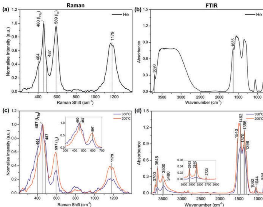
**Figure 4.2:** *In situ* (a) normalized Raman and (b) FTIR spectra of ceria rods in He flow at room temperature (black spectrum). *In situ* (c) Raman and (d) FTIR spectra of ceria rod in He flow at 200°C (red spectrum) and 350°C (blue spectrum).
