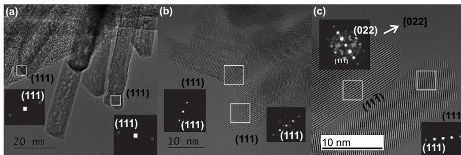
**Figure 2.8:** AC-TEM images of CeO<sub>2</sub> rods at two different magnifications [(a) and (b)]. Insets in the figures are FFTs of the boxed region in the images. (c) The lattice fringes confirm that the surfaces are {111} and the growth direction is  $\langle 110 \rangle$ . The other images likewise show only {111} surface facets.
