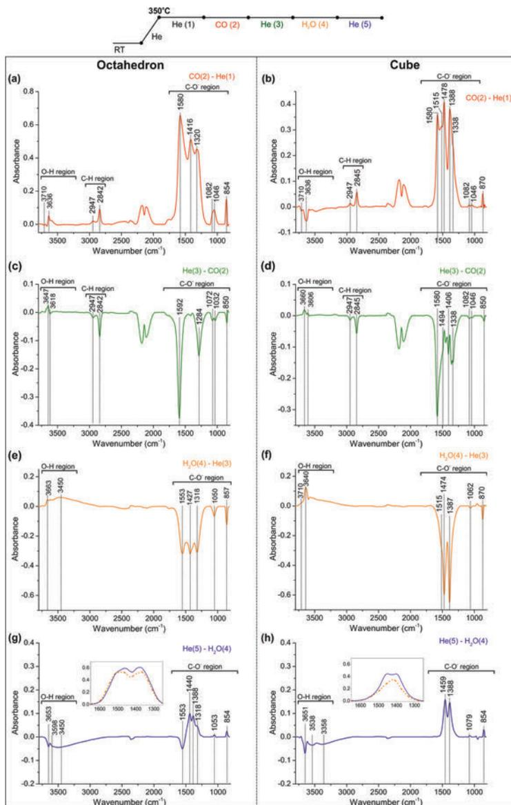
**Figure A5.6:** *In situ* FTIR subtracted spectrum at 350°C of unreduced ceria octahedra (left plots) and cubes (right plots) obtained by subtracting (a) and (b) He(1) from CO(2); (c) and (d) CO(2) from He(3); (e) and (f) He(3) from H<sub>2</sub>O(4); (g) and (h) H<sub>2</sub>O(4) from He(5). Insets in figure 5.4g and 5.4h are expanded spectra of carbonate regions obtained in H<sub>2</sub>O (dash-dotted orange) and He (5, blue) flow.
