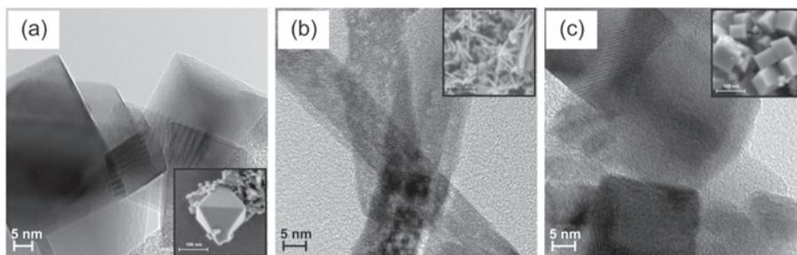
**Figure 3.1:** TEM and HRSEM (inset) images of the CeO<sub>2</sub> octahedra (a), wires (b) and cubes (c).
