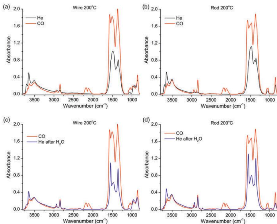
**Figure A6.1:** *In situ* FTIR spectra at 200°C of ceria wire (a, c) and rod (b, d) in He flow (black spectrum), followed by CO (red) and finally in He after regeneration in H<sub>2</sub>O vapor (blue spectrum).
