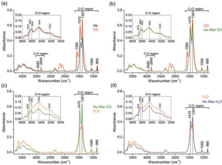
**Figure A5.5:** *In situ* FTIR spectra at 350°C of reduced ceria cubes in a) He(1, black spectrum), followed by CO(2, red line); b) CO(2) followed by He(3, green spectrum); c) He(3) followed by H<sub>2</sub>O/He(4, orange line); d) in H<sub>2</sub>O(4) followed by He(5, blue spectrum).
