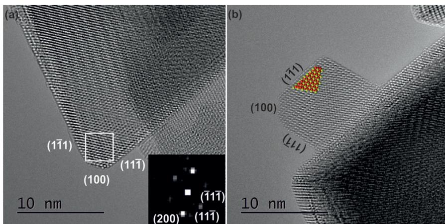
**Figure 2.5:** Aberration-corrected TEM images of large (a) and small (b)  $\text{CeO}_2$  octahedra. These expose the (111) facets and very small (100) facets. The surface termination is abrupt, and there is no amorphous layer or surface roughness present. The inset in (b) shows the structure of the  $\text{CeO}_2$  lattice (Ce atoms: green; O atoms: red) and the agreement between the white dots and the Ce atom columns.
