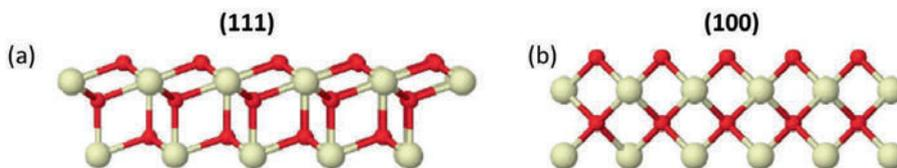
**Figure A5.10:** The ball and stick model of the (111) and (100) surfaces. Key: Ce (Light yellow) and O (red) atoms. These structures were drawn using Jmol (an open-source Java viewer for chemical structures in 3D; <http://www.jmol.org/>).
