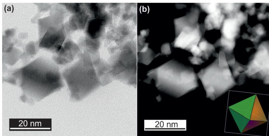
**Figure 2.3:** (a) BF and (b) HAADF STEM images showing the octahedral shapes. The thickness variation leads to the observed contrast change in the HAADF image (right), confirming the octahedral shape, as the center is thicker compared to the top and bottom (as seen from the inset). The smaller particles also expose the same dominant  $\{111\}$  surface, which is seen more clearly in the higher magnification images shown in figures 2.3 and 2.4 and figures A2.2 and A2.3 in the Appendix.
