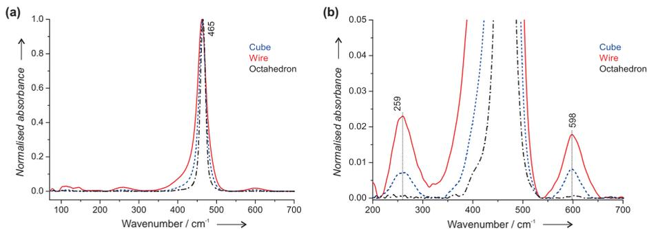
**Figure 3.3:** (a) Raman spectra (532 nm at 2 mW) of ceria cubes (dashed blue), wires (solid red) and octahedra (dash-dotted black) obtained at room temperature in air, normalized to the main peak at  $465\text{ cm}^{-1}$ ; (b) magnification of the wave number range  $200 - 700\text{ cm}^{-1}$ .
