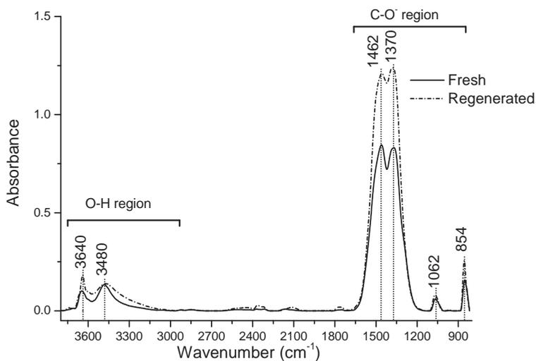
**Figure A4.8:** *In situ* FTIR spectra of ceria rods at 350°C in He flow for fresh sample (solid spectrum) and after regeneration with H<sub>2</sub>O (dash-dotted spectrum).
