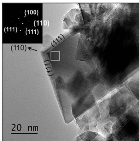
**Figure A2.3:** AC-TEM image shows that the smallest particles as well as the larger ones exhibit well-defined facets with smooth surfaces. These particles all expose prominent (111) surface facets and the (110) facet is missing, and instead we see a sharp corner.
