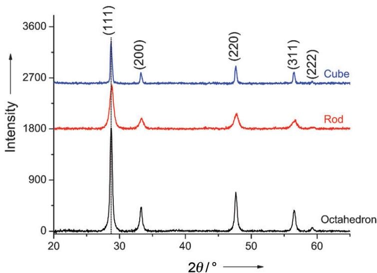
**Figure 2.1:** XRD patterns for controlled-morphology CeO<sub>2</sub> powders used in this study. The (111) reflection is highlighted with a vertical line and shows that the rods and octahedra samples have very similar lattice constants. The Appendix (figure A2.1) presents an expanded view of the (311) reflection of these samples, showing the asymmetry in peak shape (related to bimodal particle size distribution) more clearly.
