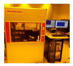
During the assignment pattern-generation in various photoresists needs to be optimized. Aspects such as 1:1 translation from design-dimensions to realized dimensions have to be studied, as well as verticality of the sidewalls of patterns in photoresist. Moreover, the type of substrate onto which the resist is coated might be of influence on the writing results.
