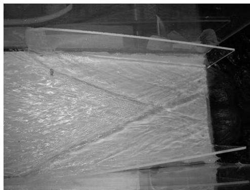
Figure 2: Left: numerical simulation of flow in a channel with a contraction. Right: Experiments (courtesy Ben Ackers).
