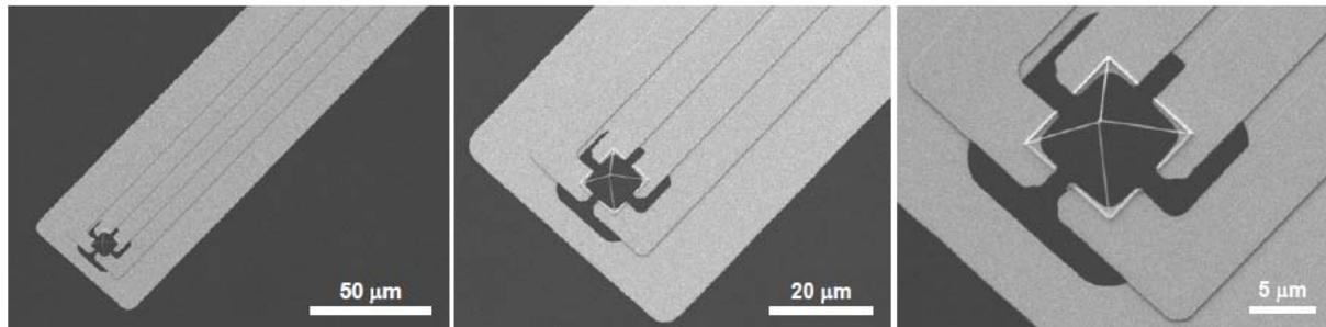
*Figure 1: SEM micrographs of a novel scanning probe designed for thermal and magnetic imaging. The probe consists of a cantilever with a pyramidal tip composed of four freestanding nanowires. The nanowires, made of a 140 nm thick silicon nitride core coated by Ti/Au layers (6 nm/30 nm), form an electrical junction at the apex of the tip. The nanowire cross junction can be addressed through the electrodes integrated on the cantilever.*
