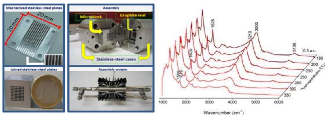
**Figure 1:** Microreactors systems (left) and operando IR spectroscopy of catalysts at high-pressure and high-temperature (right).
