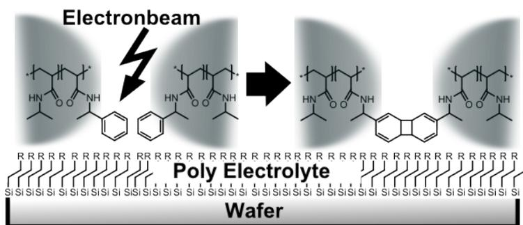
**Figure 1:** Schematic drawing of the principle of electron-beam-cross-linking between two functionalized microgel particles adsorbed at a surface.
