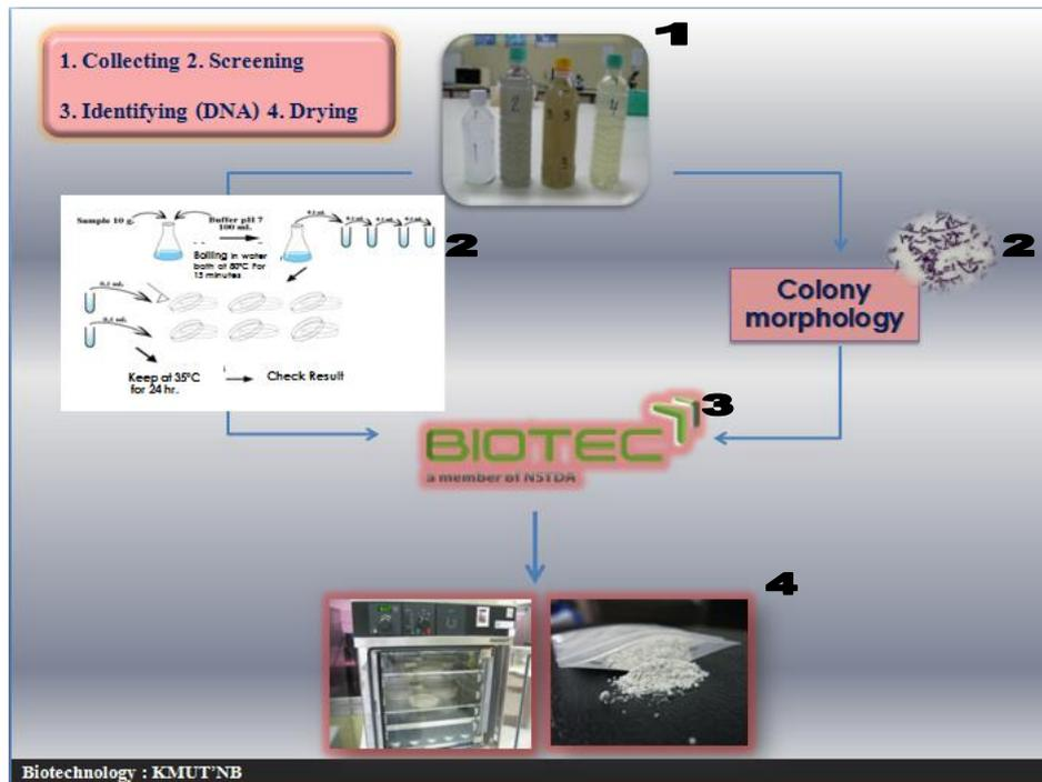
**Figure1** The process of screening and isolation EM (*B. subtilis*)
