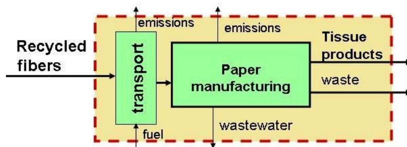
**Fig. 3.** Life cycle of tissue products from recovered fibre
