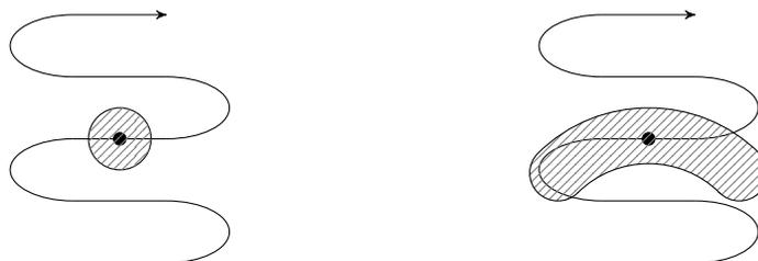
(a) Measurement noise cloud using GPS      (b) Measurement noise cloud using radar
