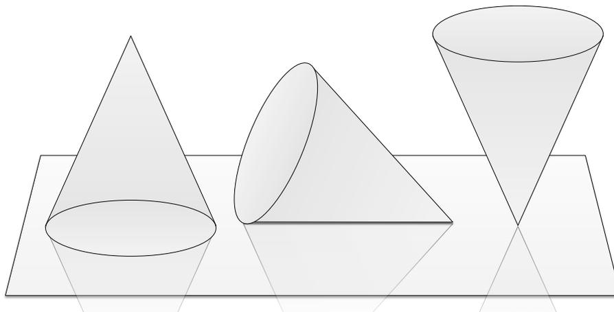
Figure 4.1: Asymptotic stability (left), neutral stability (centre), and instability (right) of a cone on a flat surface.
