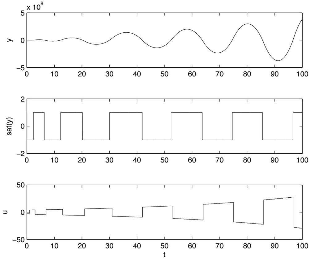
Figure 3.5: Response of the actual output, saturated output and input of the system (3.25) to Kreisselmeier's algorithm with initial conditions (3.27).
