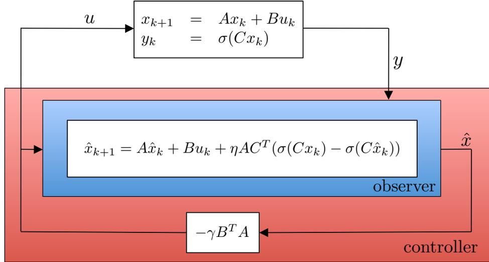
Figure 4.6: The closed-loop system (4.109)-(4.111)
