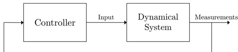
Figure 1.1: Structure of an automatic control system.
