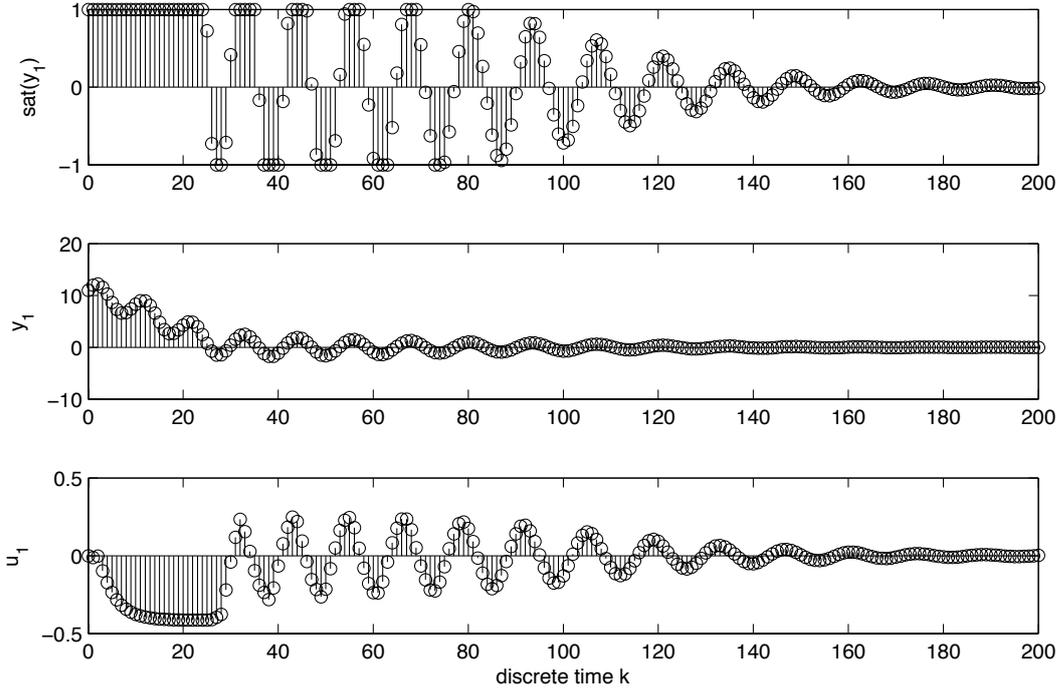
Figure 4.7: Saturated output, actual output and input of the neutrally stable system (4.122) in closed-loop with the stabilising controller.
