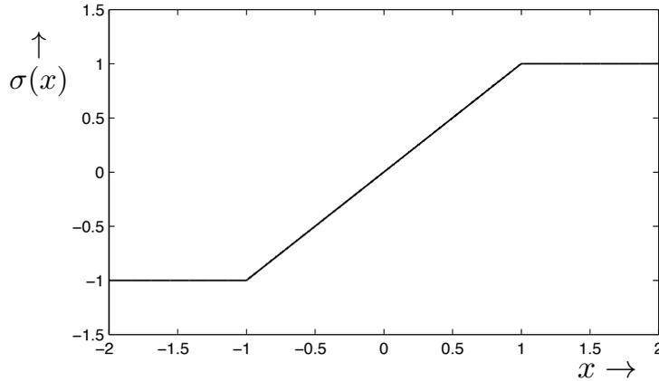
Figure 3.1: The saturation function (3.1)
