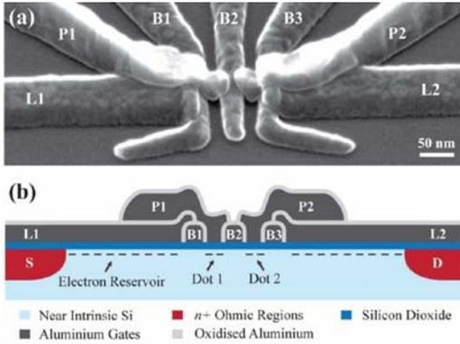
*Fig.: Scanning electron microscope image (top) and a schematic side-view (bottom) of a 3-layer silicon double quantum dot. A two-dimensional electron gas (2DEG) at the Si/SiO<sub>2</sub> interface is induced by the lead gates L1 and L2. By locally depleting the 2DEG - using barrier gates B1, B2, and B3 - two quantum dots are formed between the barriers.*
