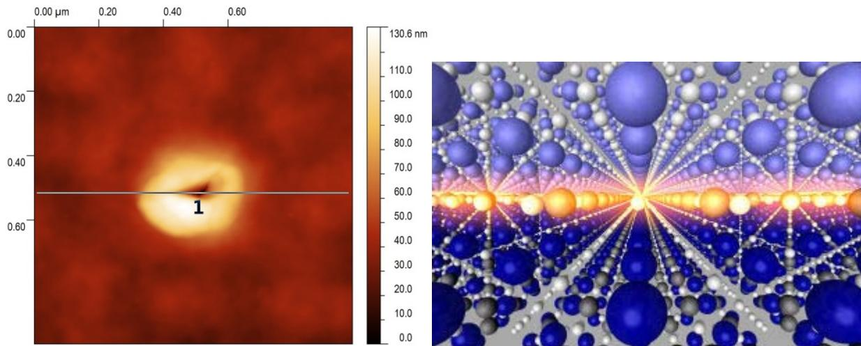
*Nano-indentation created by point-and-shoot AFM technique, enabling creation of nanoscale devices. Courtesy Bojian Xu, NE group.*
