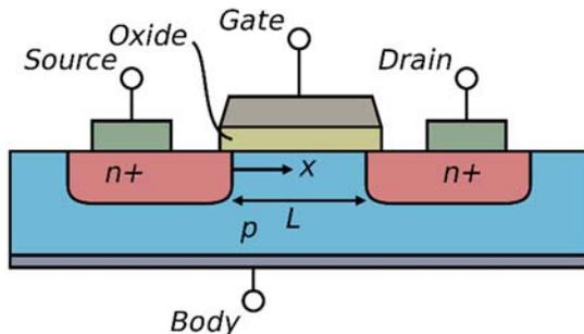
*Schematic of a classic MOSFET transistor.
