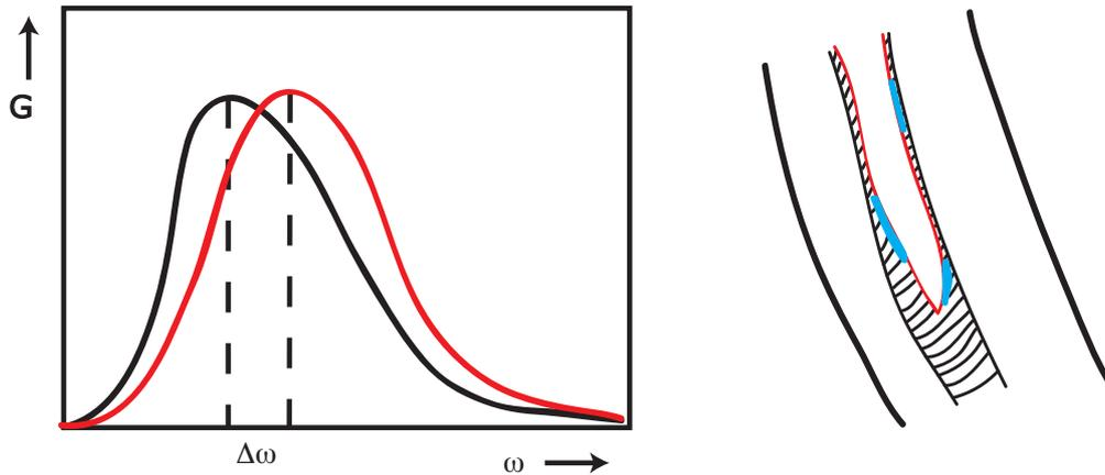
Figure 2: Indication of a shift  $\Delta\omega$  in the frequency dependency of the transfer function  $G$  in case of an affected hip replacement (red curve) compared to the desired situation (black curve). On the right a sketch is given of part of the upper leg with a metal pin (red) inserted in the remaining bone (hatched area). In blue an indication of affected bone tissue is given arising from inflammation, causing the differences in frequency response.
