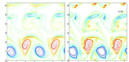
Figure 2: The potential vorticity field for the shallow water system, as computed by a high order 'conventional' method as a reference (left) and by HPM (right), see [2].
