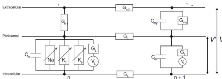
Figure 2: equivalent electrical circuit network of node in a nerve fiber
