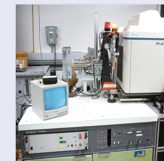
Replacement of Rigaku RU-200 generator in Boulder, USA
