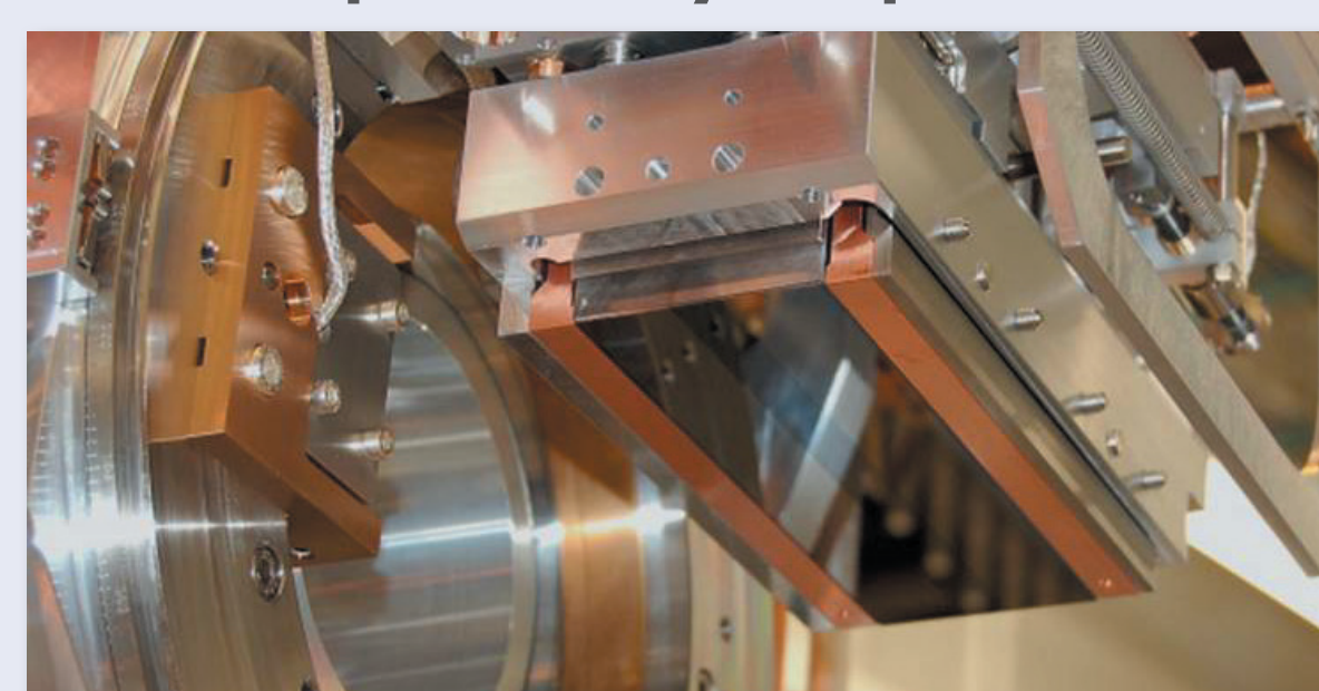
Three-stripe multilayer optics for tomographic microscopy and coherent radiology (TOMCAT at SLS; M. Stamparoni, PSI).
