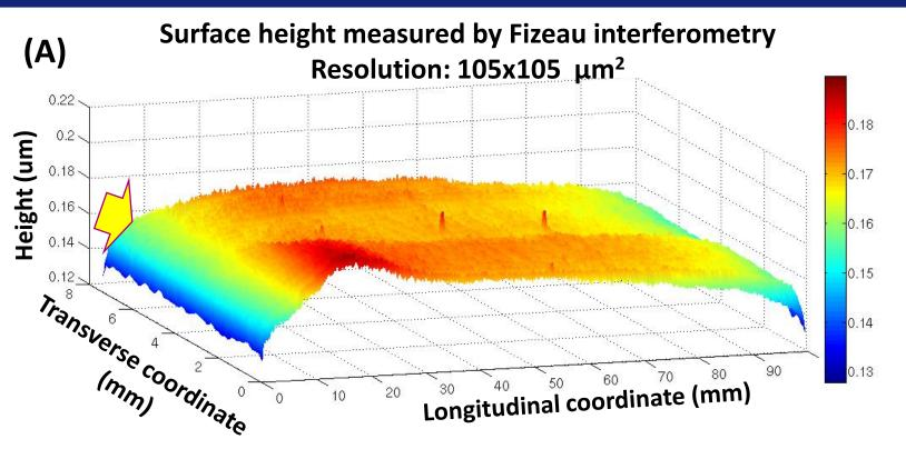
(A): Height deviation surface map of a 4 nm period  $[W/B_4C]_{60}$ multilayer measured by Fizeau interferometry. (B1) and (B2): calculated intensity and phase map from metrology data right at the multilayer stack exit.
