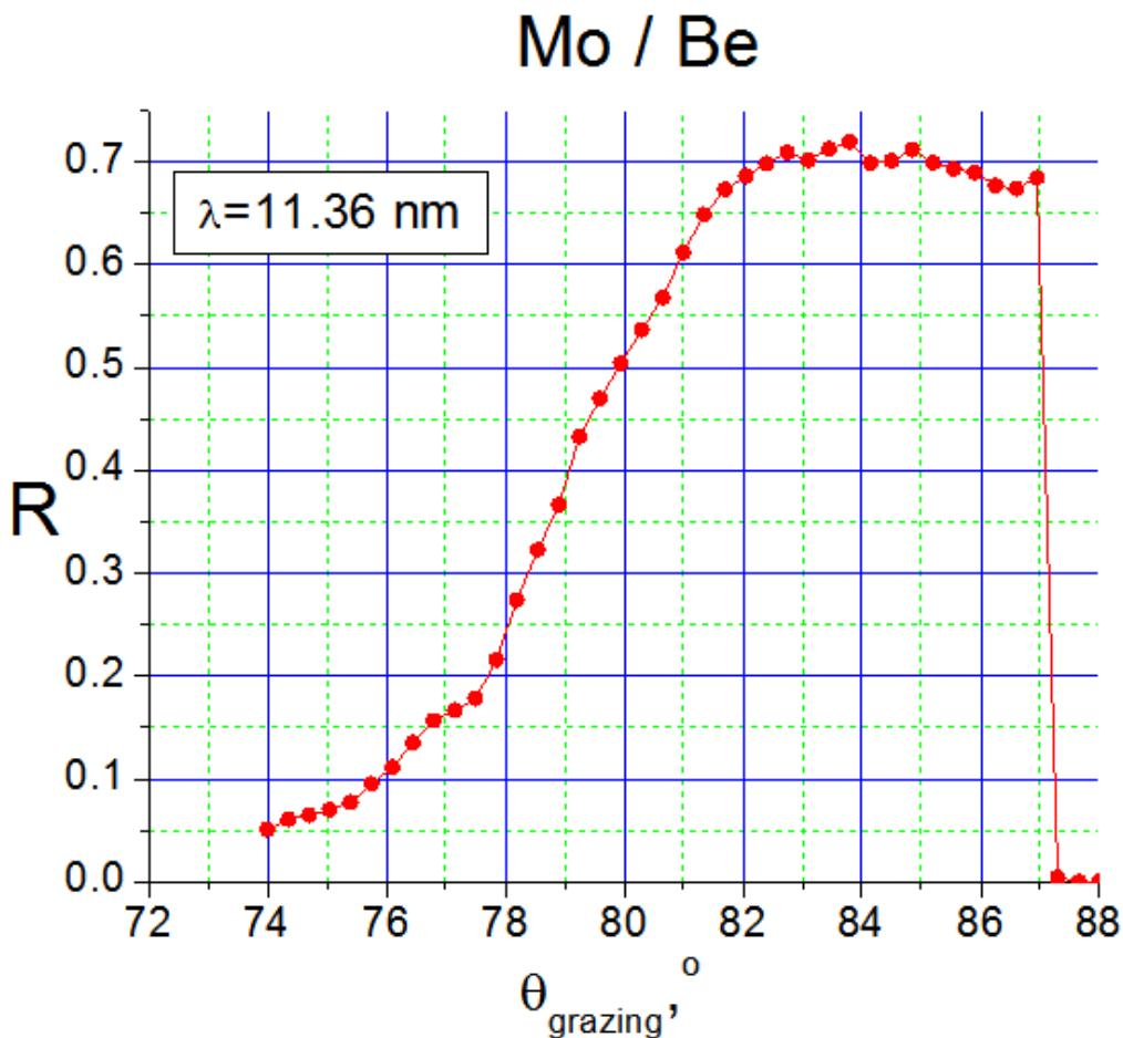
We obtain routinely reflection coefficients of Mo/Be MLM in the spectral range 11.3-11.4 nm at normal incidence reflection coefficients of 70 – 71 %
