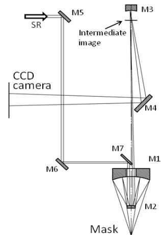
Fig. 1. A schematic of the EUV microscope: Three mirrors (M1-M3) act as a two-stage imaging system.
