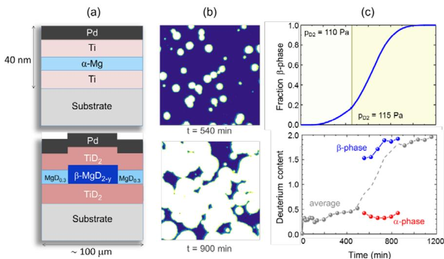
**Figure 1** (a) The magnesium-based thin film system under investigation (top) in the virgin state and (bottom) during hydrogenation. (b) Top view optical transmission images at two moments in time. The  $\beta$ -MgD<sub>2-y</sub> domains show up as bright spots that grow radially outwards. (c, top) Fraction of  $\beta$ -MgD<sub>2-y</sub> as a function of time as determined from the optical transmission images. (c, bottom) deuterium content of the Mg layer, as determined by neutron reflection.
