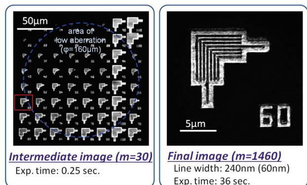
Fig. 2. At-wavelength images of EUV lithography mask.
