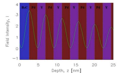
Simulation of the electric field of the same sample described above under 10keV irradiation. Grazing incident angle is set at its Bragg angle.
