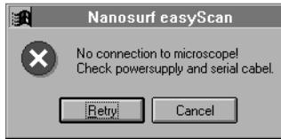
By pressing 'Cancel' a simulation of the microscope is started. This imitates most of the functions of the real microscope. The sample is replaced by a mathematical description of an atomic arrangement.
