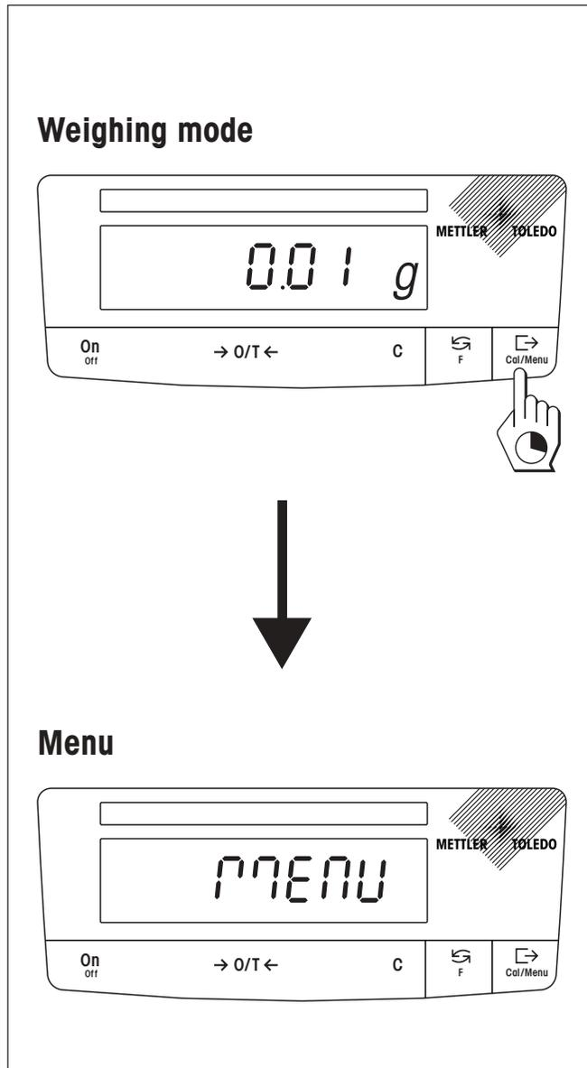
The balances have two operator control levels: the **weighing mode** and the **menu**. The function of each individual key depends on the operator control level and how long the key is pressed.
