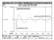
Rapid changes to measurement values can be recorded with METRAHit®22M/26M and 29S instruments at sampling rates of 1 kHz and 2 kHz respectively.
