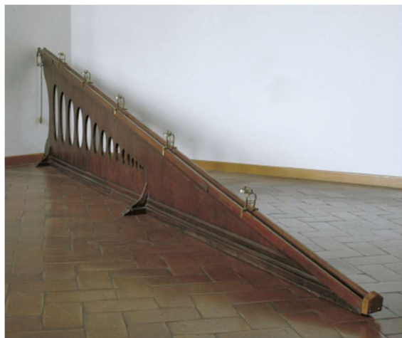
Figure 1 Experimental device of Galileo Galilei for experiments of the law of falling bodies. In rolling down the inclined plane, the ball hits the bells which are attached following a quadratic law. This device is rebuilt in Florence. (Frauenberger, 2007)
