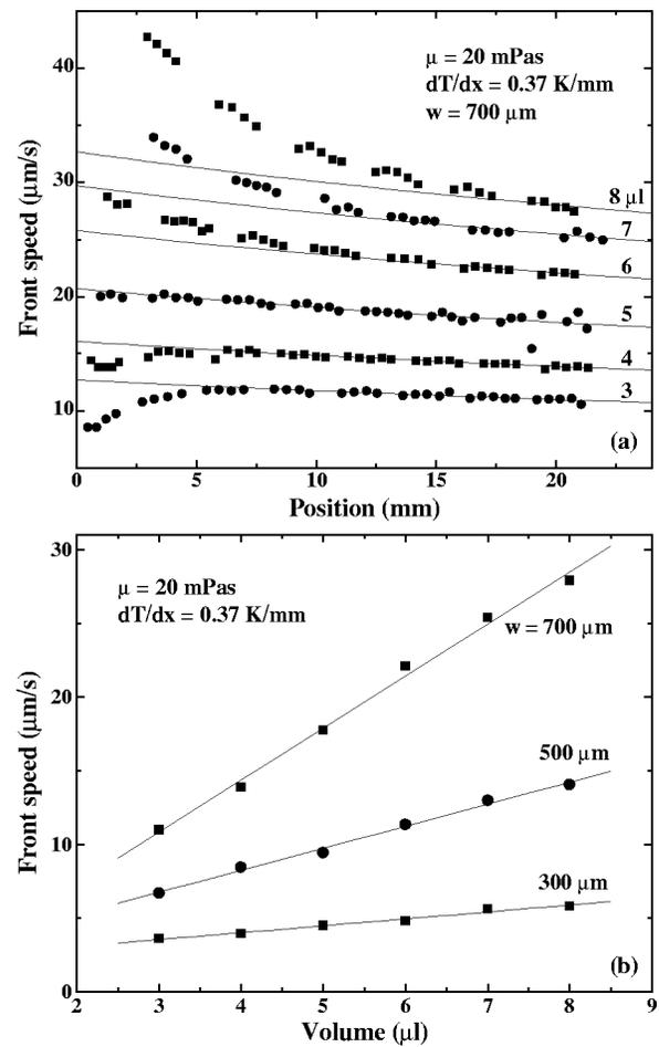
FIG. 6. (a) Position dependence of the liquid front speed for  $w = 700 \mu\text{m}$ ,  $|dT/dx| = 0.37 \text{ K/mm}$  and  $V$  ranging from 3 to 8 μl. The solid lines correspond to the constant flux solution given by Eq. (19). (b) Volume dependence of the front speed for stripe widths  $w = 300, 500$  and  $700 \mu\text{m}$  at  $x = 20 \text{ mm}$ . The solid lines represent linear fits to the experimental data.
