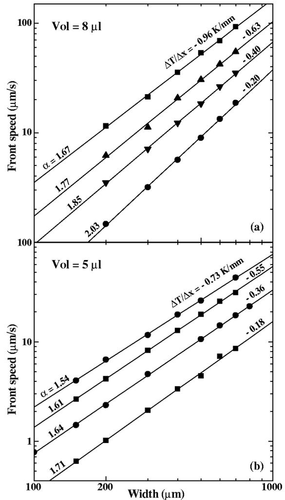
FIG. 8. Liquid front speed as a function of the stripe width for (a)  $V=8 \mu\text{l}$  and (b)  $V=5 \mu\text{l}$  at  $x=18 \text{ mm}$ . The data are well represented by power law relations  $u \sim w^\alpha$  (solid lines). The exponent  $\alpha$  ranges from 2 for small gradients and larger volumes to  $3/2$  for large gradients and smaller volumes.
