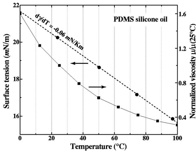
FIG. 2. Temperature dependence of the surface tension  $\gamma$  and normalized viscosity  $\mu/\mu(25^\circ\text{C})$  for PDMS (Refs. 21, 22).  $d\gamma/dT$  is essentially constant for the temperature range of the experiments (20 to 60  $^\circ\text{C}$ ).
