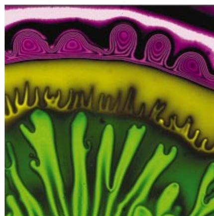
FIG. 2. A droplet of glycerol containing SDS spreading on a glycerol film. The images were recorded 5542 and 11 565 s after droplet deposition. Vertical image dimension=1 cm.
