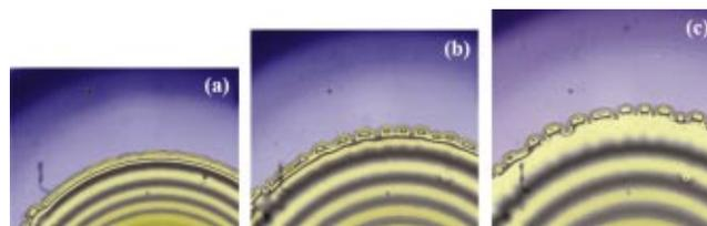
FIG. 3. A droplet of PDMS spreading on a tetra(ethylene glycol) film. The images were recorded at (a)  $t=2611$ , (b) 3811, and (c) 5011 s after droplet deposition. Lateral image dimension=1 cm.
