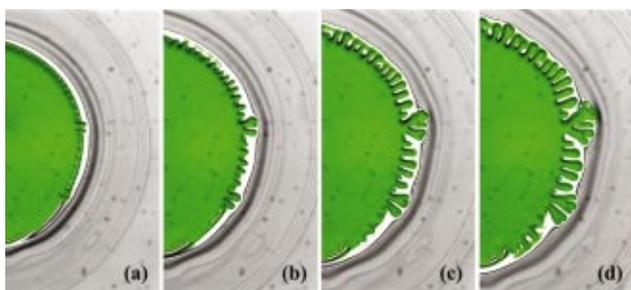
FIG. 1. A droplet of glycerol containing sodiumdodecylsulfate spreading on a glycerol film. The images were recorded at (a)  $t=20$ , (b) 28, (c) 36, and (d) 44 s after droplet deposition. Vertical image dimension=1 cm.
