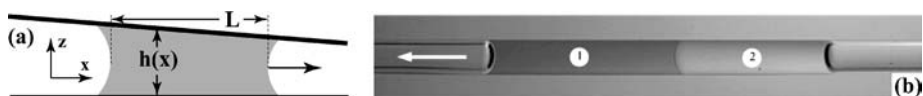
Figure 4 (a) A liquid plug with \theta < 90^\circ ( \theta > 90^\circ ) moves toward (away from) the narrow gap region. (b) A self-propelled bislug ( \gamma_{12} = 18.0 mN/m) of ethylene glycol ( \gamma_1 = 47.7 mN/m) and silicone oil ( \gamma_2 = 20.3 mN/m) in a 1 mm diameter glass capillary. [Reprinted from Bico & Quéré (2002) with permission from Cambridge Univ. Press.]
