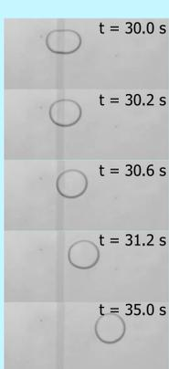
◀ The drop can be held in the trap for analysis, and released to go to the next position. Different electrode configurations can be used to guide the drop as well.
