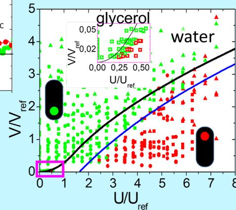
Rescaled trapping diagram. The lines give the predicted transition depending on how the pinning is reduced by electrowetting. Inset: zoom on glycerol:water droplets
