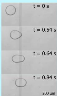
◀ Shows a water drop in oil flow. The pinning force exceeds the viscous drag.
