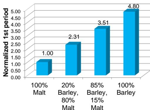
Figure 2: Normalized filterability of the different trials. In the case of 100% barley, the 1<sup>st</sup> period is estimated to 32 hours.
