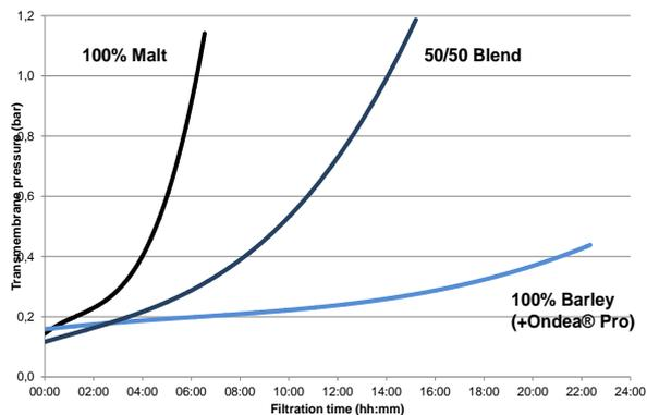
Figure 1: Filtration data from a 1 hl BMF pilot plant of 100% malt, 100% barley and a 50/50 blend of the two.
