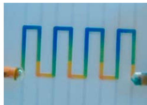
Figure 3: Switching pH gradients in microchannels.
