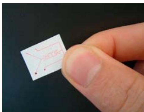
Figure 1: Porous microfluidic chip made by phase separation micromolding.
