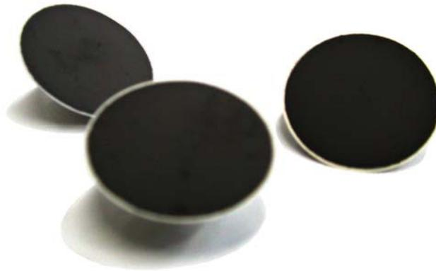
*Symmetric cells of LSCM on a TZ3Y electrolyte*
