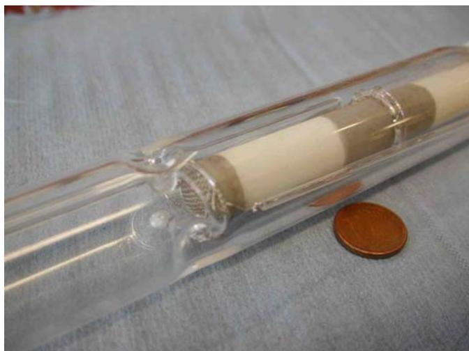
**Figure 9: Picture of oxygen sensor and pump in quartz tube.**
