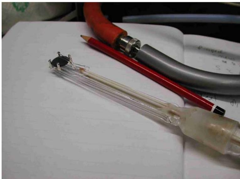
**Figure 14:** Second sample holder (S2) with sample. The arms are connected close to the glass joint. The 4-bore alumina tube (white) is in the middle of the sample holder.
