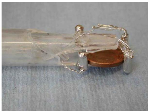
**Figure 11:** Sample holder tip with 4 electrodes. The inner quartz tube is pressed slightly, with the spring, to the left. The two electrodes on the right are connected on the inner quartz tube. These two electrodes press the 1 euro cent against the other two electrodes that are fixed on the outer quartz tube.
