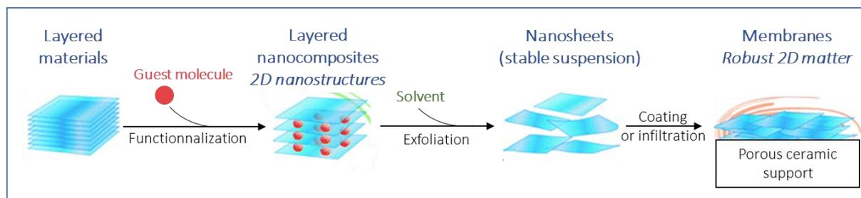
Figure 1. Overview of typical nanosheet-based membranes and their preparation routes.
