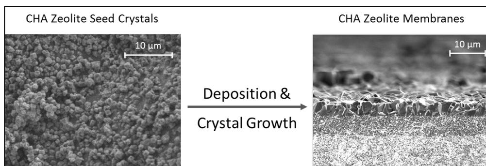
Figure 1: The SEM images of the CHA seed crystals (on the left) which are further deposited on a porous support and grown into a continuous zeolite membrane layer
