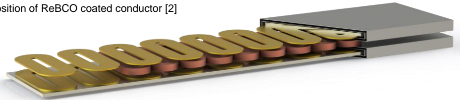
Composition of ReBCO coated conductor [2]
