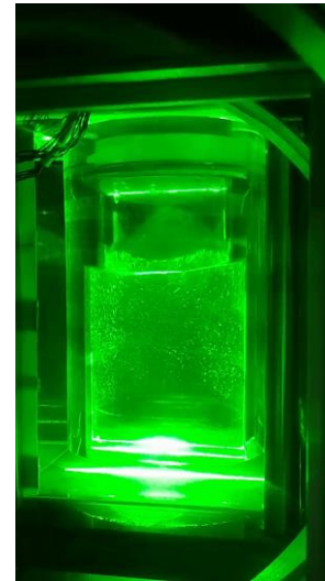
2D Particle Image Velocimetry sloshing test
