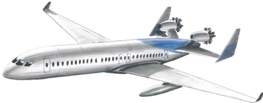
Figure 5. A Multi-Fuel A320 class of aircraft with podded LNG tanks and open rotors designed by a DSE group.
