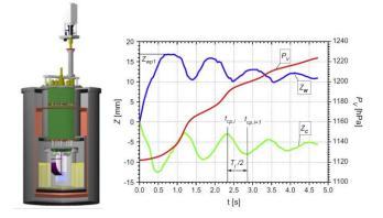
Figure 1: Experimental setup, plots of the vapour pressure, the positions of the center point and the contact line at the wall [1].
