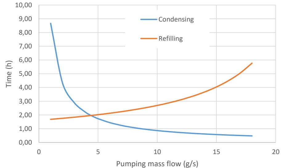
$$t_{liquefaction} = \frac{V_{cryostat} \cdot \rho_{sat\ GHe\ @\ 1.3\ bar} \cdot L_{@\ 1.3\ bar} \cdot (1 - \%_{cryostat\ initial\ filling})}{\dot{m}_{pumping} \cdot L_{@\ 30\ mbar} \cdot (1 - \%_{flash})}$$
