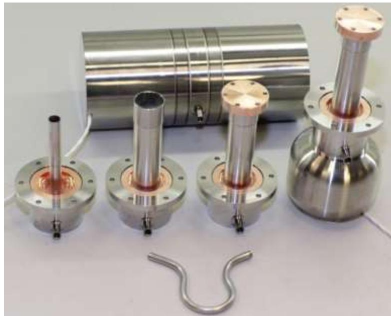
Implementation of heat exchangers in PT coolers is “easier” due to mass flow through heat exchangers. Copper slit heat exchangers (EDM machining) are being used.
