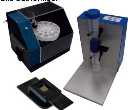
Figure 1 ASCD, pump with disposable filtration unit and staining holder with microsieve slide for detection of CTC discarded by the CellSearch system
