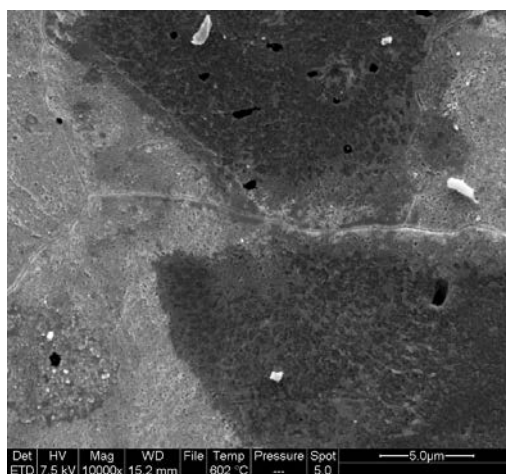
SI Movie 1: ESEM movie showing carbon precipitation on the surface of the Ni foam after prolonged exposure at 600 °C of the reduced Ni foam to C 2 H 4 and H 2 at pressures between 10 -2 Pa and 100 Pa followed by decreasing ethylene pressure to below 10 -2 Pa
